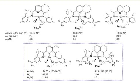
Chart 2 Comparison of catalytic activity and polymer properties displayed using Fe1 and Fe4 with structurally related Fe<sub>7a</sub><sup>8b</sup> Fe<sub>7b</sub><sup>8c</sup> and Fe<sub>2,6-diPr</sub>, in each case activation with MMAO at  $P_{C_2H_4} = 10$  atm.
