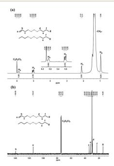
Fig. 8 For the polyethylene obtained using Fe7/MAO at 100 °C, (a) the  $^{1}$ H NMR spectrum, including an expansion of the vinylic region, and (b)  $^{13}$ C NMR spectrum (entry 21, Table 4); both recorded in tetra-chloroethane- $d_2$  at 100 °C.
