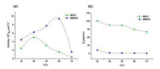
Fig. 6 For Fe5/MAO and Fe5/MAO, comparison of (a) activity versus reaction temperature and (b) polyethylene molecular weight versus reaction temperature.
