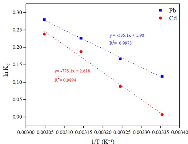
Fig. 8 Van 't Hoff plot used to obtain the adsorption thermodynamic parameters of Pb(II) and Cd(II) on cement kiln dust (CKD): linear fits of  $\ln K_d$  versus  $1/T$  (K<sup>-1</sup>) were used to obtain  $\Delta H^\circ$  from the slope  $-\Delta H^\circ/R$  and  $\Delta S^\circ$  from intercept  $\Delta S^\circ/R$ . The corresponding regression equations and  $R^2$  values are also shown.
