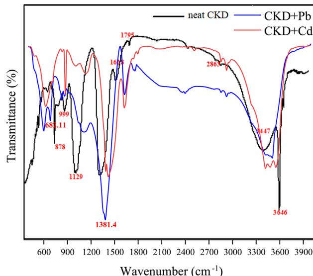
Fig. 1 FTIR spectra of the neat CKD and CKD loaded with Pb and Cd metals.
