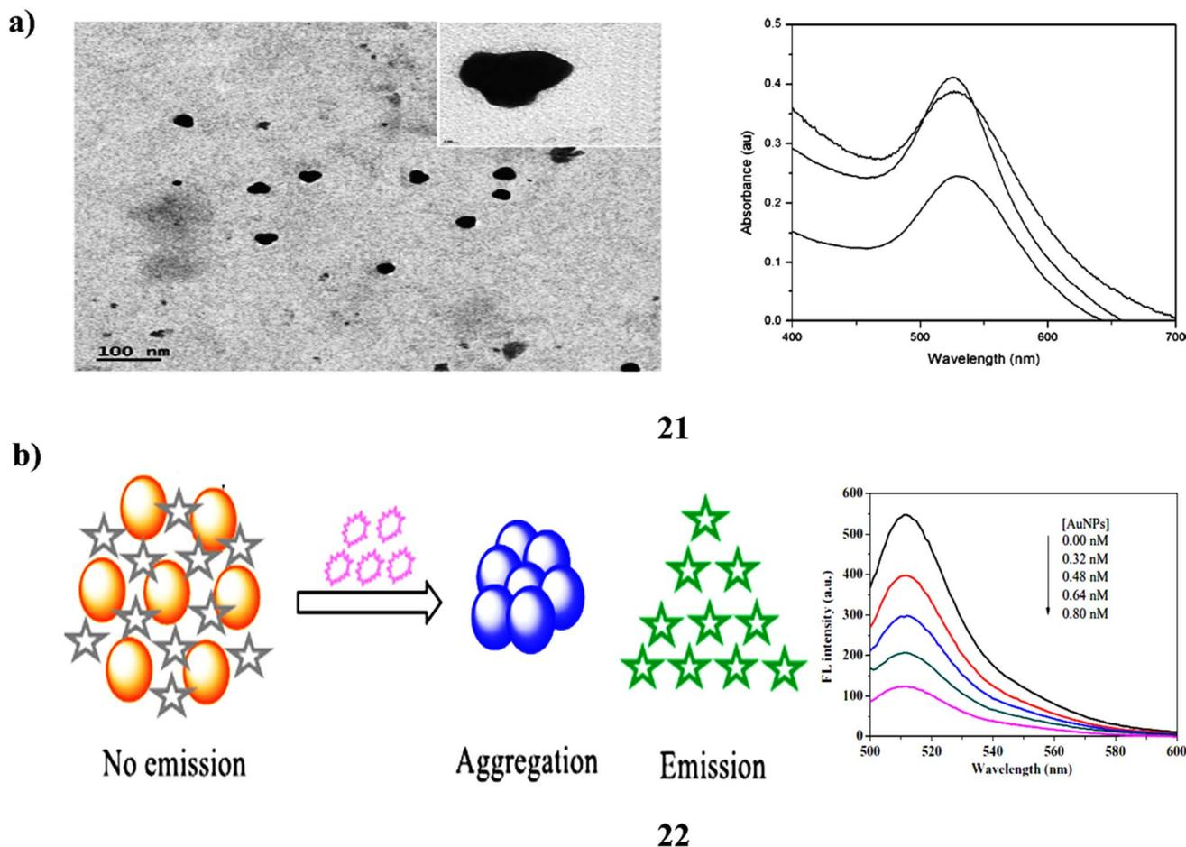
Fig. 12 (a) Photophysical response of green-synthesized fluorescein-AuNP nanofluids (21) reproduced from ref. 40 with permission from Elsevier Publisher, Copyright 2016. (b) Fluorescent sensing of bi thiols using fluorescein-AuNP probes (22) reproduced from ref. 41 with permission from Elsevier Publisher, Copyright 2020.
