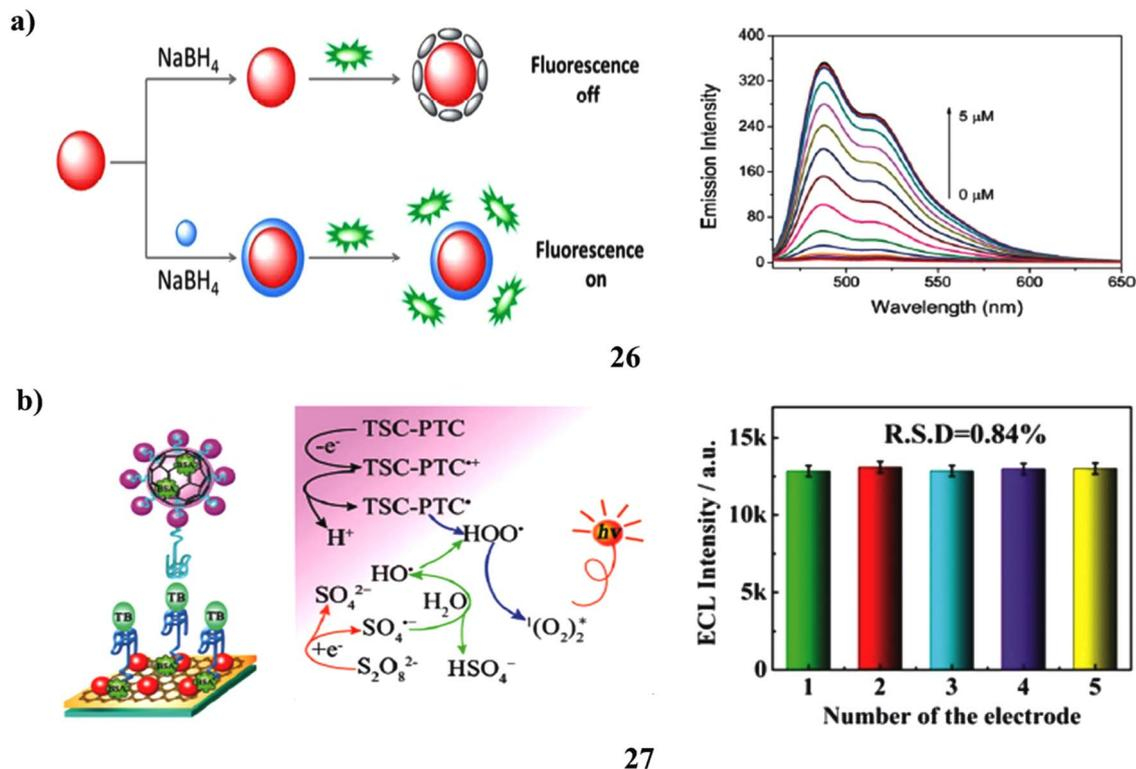
Fig. 15 (a) Fluorescence recovery assay for  $\text{Hg}^{2+}$  detection using perylene-AuNP nanoprobes (26) reproduced from ref. 45 with permission from Royal Society of Chemistry Publisher, Copyright 2016. (b) Electrochemiluminescence study of PTCA-TSC-C60-AuNP composite for thrombin sensing (27) reproduced from ref. 46 with permission from Royal Society of Chemistry Publisher, Copyright 2015.
