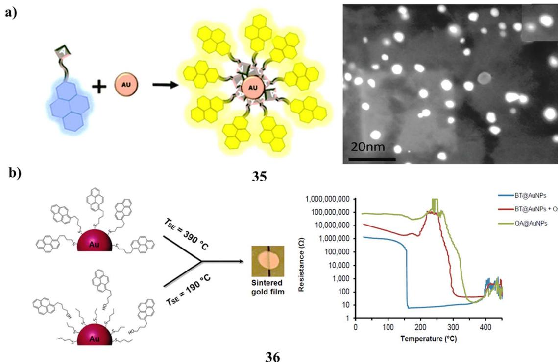
Fig. 20 (a) Excimer emission behavior of pyrene-adenine-AuNPs (35) reproduced from ref. 54 with permission from Royal Society of Chemistry Publisher, Copyright 2021. (b) Thermal stability of pyrene-butanethiol-AuNPs under sintering conditions (36) reproduced from ref. 55 with permission from American Chemical Society Publisher, Copyright 2017.
