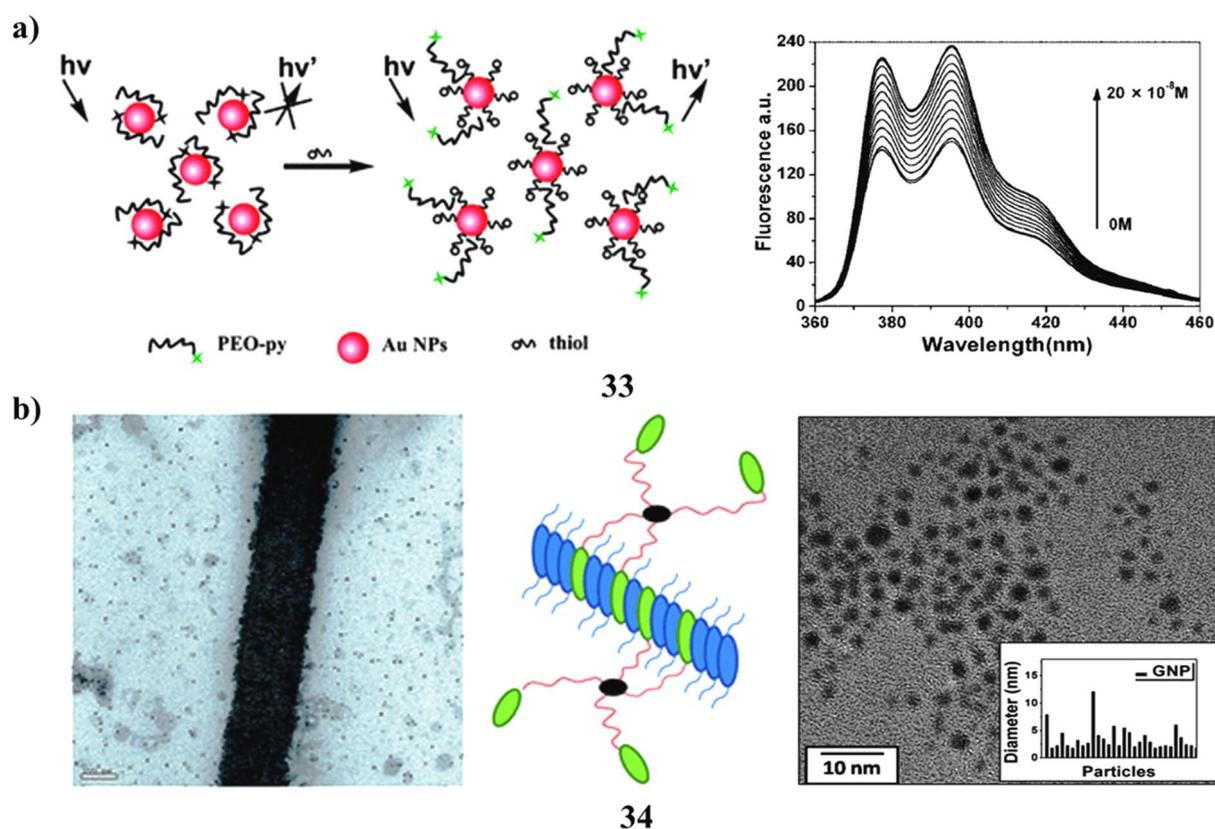
Fig. 19 (a) Fluorescence emission of PEGylated pyrene-AuNPs for bi-thiol detection (33) reproduced from ref. 52 with permission from Royal Society of Chemistry Publisher, Copyright 2010. (b) TEM morphology showing  $\pi$ - $\pi$  stacking of pyrene-thiol-functionalized AuNPs (34) reproduced from ref. 53 with permission from Royal Society of Chemistry Publisher, Copyright 2015.
