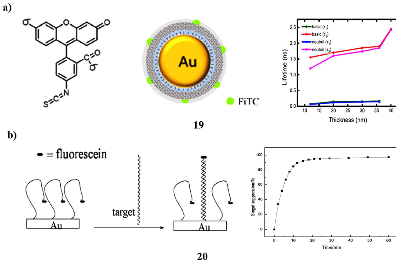
Fig. 11 (a) Fluorescence enhancement in GNP@silica@FITC core-shell systems with varied shell thickness (19) reproduced from ref. 38 with permission from Elsevier Publisher, Copyright 2021. (b) Electrochemical DNA biosensor using fluorescein-labeled AuNP electrodes (20) reproduced from ref. 39 with permission from Elsevier Publisher, Copyright 2013.
