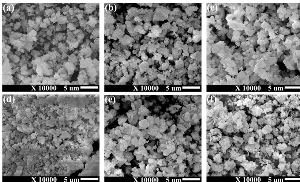
Fig. 9 Scanning electron microscopy images of synthesized  $\text{CaO}_2$  under varying synthesis conditions, defined in Table 1 (a) composite A, (b) composite B, (c) composite C, (d) composite D, (e) composite E, and (f) composite F.
