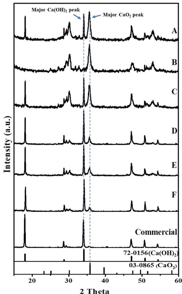
Fig. 4 XRD patterns of synthesized  $\text{CaO}_2$  composites at different  $\text{H}_2\text{O}_2$  concentrations. A ( $\text{H}_2\text{O}_2$  25%, mole ratio 1 : 1), B ( $\text{H}_2\text{O}_2$  30%, mole ratio 1 : 1), C ( $\text{H}_2\text{O}_2$  35%, mole ratio 1 : 1), D ( $\text{H}_2\text{O}_2$  25%, mole ratio 7 : 1), E ( $\text{H}_2\text{O}_2$  30%, mole ratio 8.5 : 1), F ( $\text{H}_2\text{O}_2$  35%, mole ratio 10 : 1).
