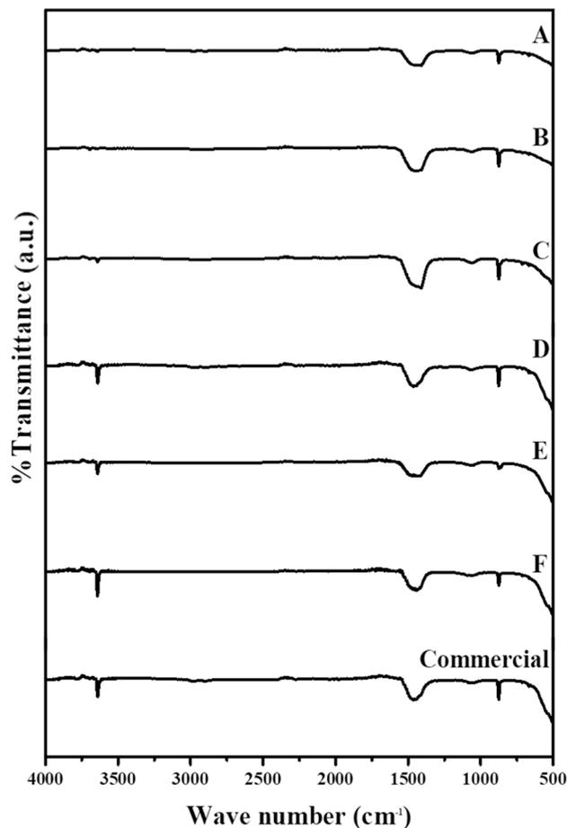
Fig. 7 Fourier-transform infrared spectroscopy spectra of synthesized  $\text{CaO}_2$  composites (see Table 1) at different  $\text{H}_2\text{O}_2$  concentrations: A ( $\text{H}_2\text{O}_2$  25%, mole ratio 1 : 1), B ( $\text{H}_2\text{O}_2$  30%, mole ratio 1 : 1), C ( $\text{H}_2\text{O}_2$  35%, mole ratio 1 : 1), D ( $\text{H}_2\text{O}_2$  25%, mole ratio 7 : 1), E ( $\text{H}_2\text{O}_2$  30%, mole ratio 8.5 : 1), F ( $\text{H}_2\text{O}_2$  35%, mole ratio 10 : 1).
