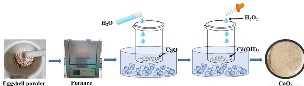
Fig. 2 Schematic diagram of calcium peroxide (CaO<sub>2</sub>) synthesis from eggshell waste.
