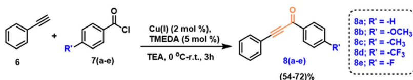
Scheme 1 (A) Synthesis of 1-methyl-1 H -indole-2-carboxamide derivatives 5(a-d). (B) Synthesis of 1,3-diphenylprop-2-yn-1-one derivatives 8(a-e).
