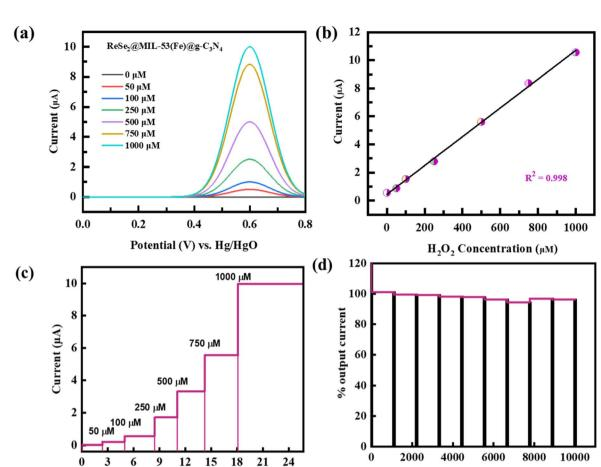
Fig. 12 (a) DPV curves at varying H<sub>2</sub>O<sub>2</sub> concentrations, (b) calibration curve, (c) chronoamperometric (CA) evaluation of the response time, and (d) stability analysis for H<sub>2</sub>O<sub>2</sub> sensing
