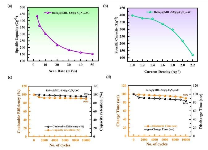
(a and b) Specific capacity measurement results from CV, and GCD plots, (c and d) stability tests of the present hybrid device.
