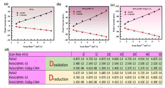
Fig. 5 Anodic and cathodic peak currents versus scan rate for the (a) ReSe<sub>2</sub>, (b) MIL-53(Fe)@ReSe<sub>2</sub>, and (c) ReMIL-CN composite material and (d) oxidation and reduction diffusion coefficients of the three materials.
