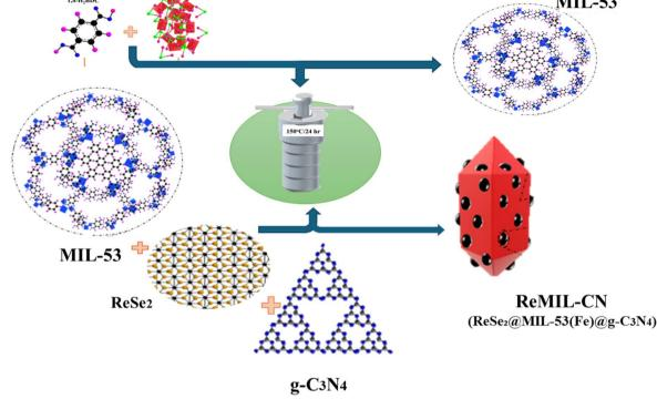
Schematic showing the integration of ReSe<sub>2</sub>, iron-MOF (MIL-53), and g-C<sub>3</sub>N<sub>4</sub> into the hybrid ternary composite material ReMIL-CN.
