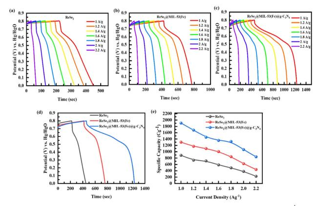
Fig. 4 GCD characteristics curves of (a) ReSe<sub>2</sub>, (b) MIL-53(Fe)@ReSe<sub>2</sub>, and (c) the ternary composite ReMIL-CN over the  $1-2.2 \text{ A g}^{-1}$  input current range, (d) comparative GCD performance of the three nanocomposites at 50 mV s<sup>-1</sup>, and (e) their measured specific capacity values.
