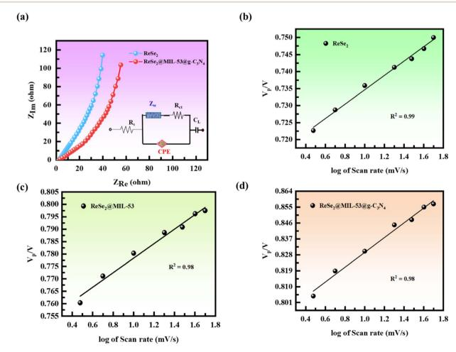
Fig. 6 (a) EIS measurement of  $ReSe_2$  and  $MIL-53(Fe)@ReSe_2@g-C_3N_4$  composite (b-d) peak voltage as a fuction of log of scan rate for  $ReSe_2$ ,  $MIL-53(Fe)@ReSe_2$ , and ReMIL-CN composite.
