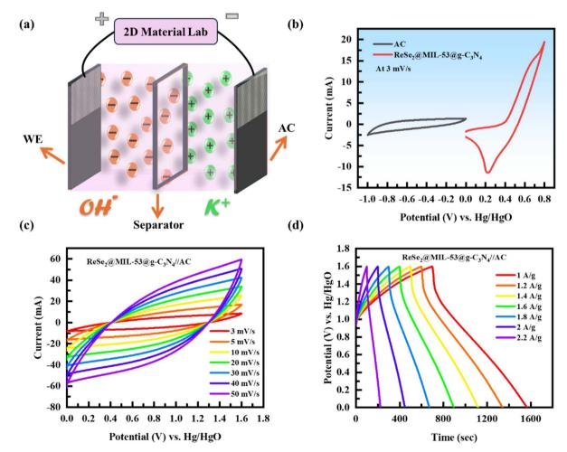
Fig. 8 (a) Real device depiction, (b) individual CV plots of the cathode and anode, and (c and d) hybrid device CV and GCD plots.
