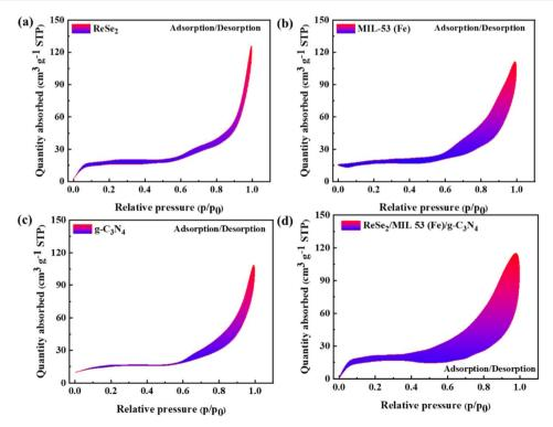
Fig. 7 BET analysis of the (a) ReSe<sub>2</sub>, (b) MIL-53(Fe), (c) g-C<sub>3</sub>N<sub>4</sub>, and (d) ReMIL-CN composite electrodes.
