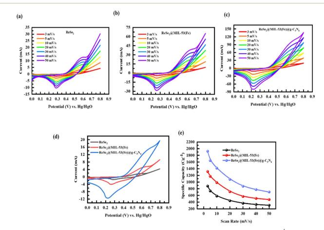
Fig. 3 CV curves of (a) ReSe<sub>2</sub>, (b) MIL-53(Fe)@ReSe<sub>2</sub>, and (c) the ReMIL-CN composite for the scan rate range of 3-50 mV s<sup>-1</sup>, (d) comparative CV performance of the three electrodes at 50 mV s $^{-1}$ , and (e) specific capacity versus scan rate for the three electrodes, calculated from CV results.
