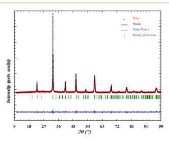
Fig. 1 Rietveld-refined X-ray diffraction patterns of La<sub>0.5</sub>Sm<sub>0.2</sub>Sr<sub>0.3</sub>-MnO<sub>3</sub> sample: the calculated data is depicted as solid black line, the observed data appeared as red dots, the Bragg reflection positions are represented by green ticks, and the blue line demonstrates the difference between the calculated and observed data
