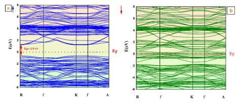
Fig. 3 Band structure (spin up (a) and down (b)) for La<sub>0.5</sub>Sm<sub>0.2</sub>Sr<sub>0.3</sub>MnO<sub>3</sub> sample.
