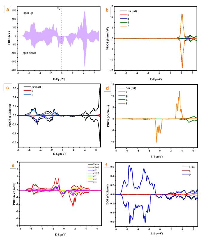
Fig. 2 (a) Total density of states for  $La_{0.5}Sm_{0.2}Sr_{0.3}MnO_3$ , (b-f) partial density of states of La, Mn 3d, Sm and O.
