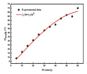
Fig. 7 Exchange field dependence of magnetization for the La<sub>0.5</sub>-Sm<sub>0.2</sub>Sr<sub>0.3</sub>MnO<sub>3</sub> sample. Red line as the fit by the equation  $H_{\text{exch}} = \lambda_1 M + \lambda_3 M^3$ .
