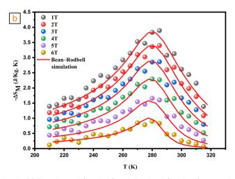
Fig. 9 (a) Experimental (symbols) and simulated (red lines) magnetization M vs.  $\mu_0H$ . (b) Experimental (symbol) and theoretical (red line) magnetic entropy change versus temperature under different magnetic fields.
