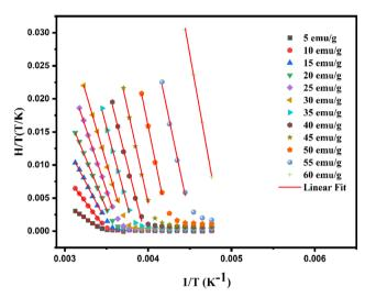
Fig. 6 Variation of H/T vs. 1/T curves with constant values of magnetization for the  $\rm La_{0.5}Sm_{0.2}Sr_{0.3}MnO_3$  sample.
