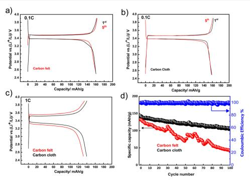
Charge/discharge profile at 0.1 C (a and b) and long-term cycling at 1 C (c and d) of carbon felt and carbon cloths current collectors.
