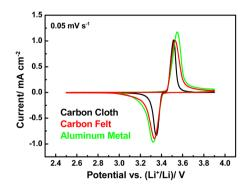
Fig. 3 Cyclic voltammetry curves of LFP based lithium slurry batteries using different current collectors.
