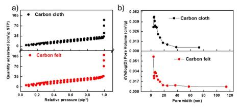
Fig. 2 N<sub>2</sub> adsorption-desorption isotherms (a) and pore size distribution (b) of carbon cloth and carbon felt current collectors.
