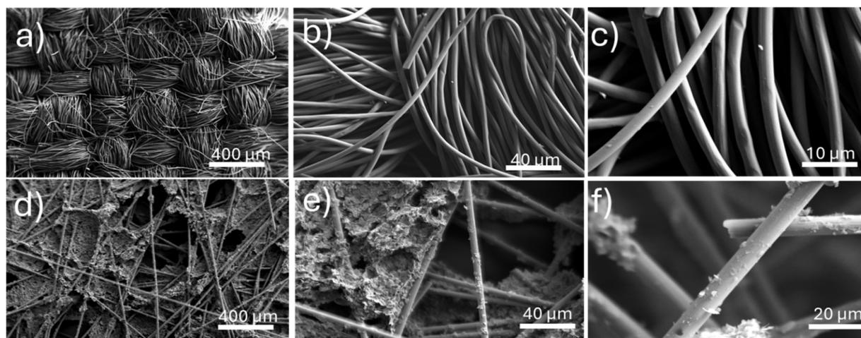
Fig. 1 SEM images of carbon cloth (a–c) and carbon felt (d–f) current collectors.
