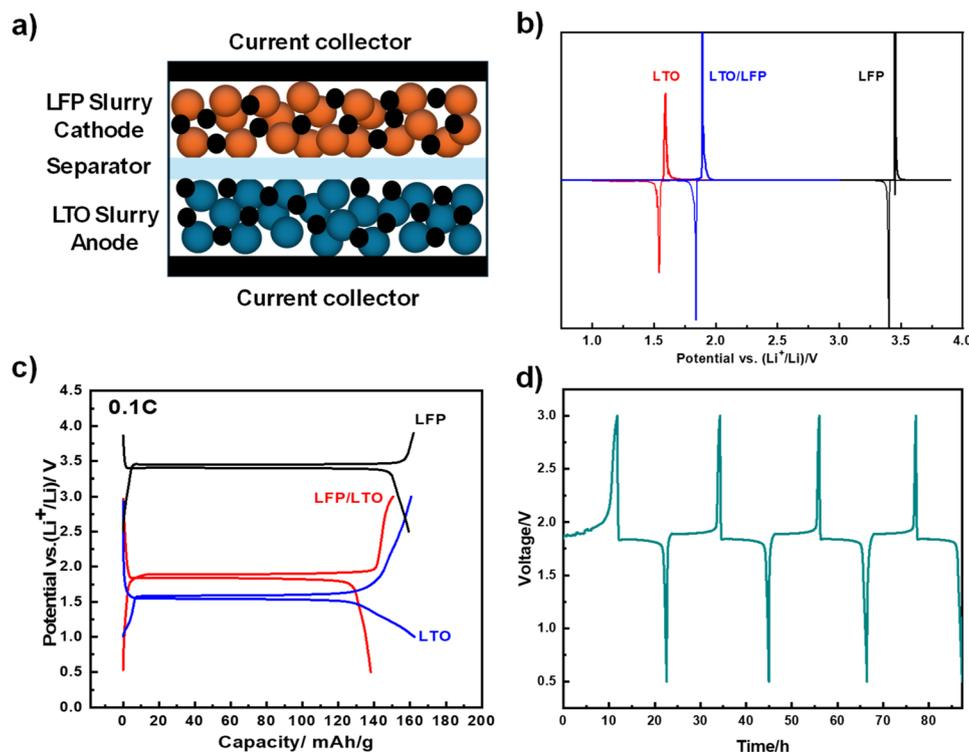
Fig. 7 Schematic illustration of the LFP based lithium slurry full cell (a). Differential capacity plots,  $dQ/dV$  vs. voltage, for the first cycle of LTO, LFP and the full cell (b). Galvanostatic charge–discharge profiles of LFP||LTO (c and d).
