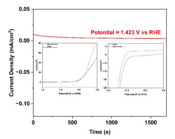
Fig. 8 Stability for Co–Ba–TPA MOF using chronoamperometry at 1.423 V vs. RHE and the inset is the LSV curves before and after 30 min test.
