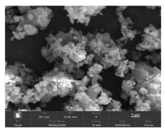
Fig. 3 SEM image of Co-Ba-TPA MOF.
