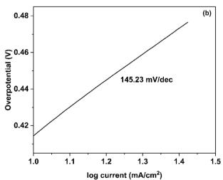
Fig. 5 (a) Polarization curve (b) Tafel plot of Co-Ba-TPA MOF for HER.
