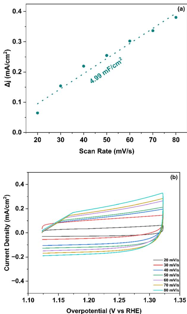
Fig. 7 (a)  $\Delta j$  plot as a function of scan rate and  $C_{\text{dl}}$  calculation (b) CV curves at various scan rates.
