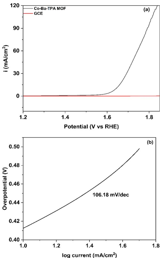
Fig. 6 (a) Polarization curve (b) Tafel plot of Co–Ba–TPA MOF for OER.
