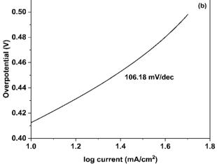
Fig. 6 (a) Polarization curve (b) Tafel plot of Co-Ba-TPA MOF for OER.
