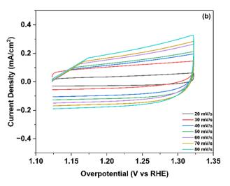
Fig. 7 (a)  $\Delta j$  plot as a function of scan rate and  $C_{\rm dl}$  calculation (b) CV curves at various scan rates.
