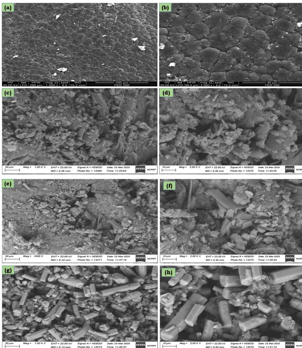
**Fig. 3** SEM images of synthesized samples at different magnifications: (a) CH at  $1000\times$ , (b) CH at  $3000\times$ , (c) CH-DEPS 1 at  $1000\times$ , (d) CH-DEPS 1 at  $2000\times$ , (e) CH-DEPS 2 at  $1000\times$ , (f) CH-DEPS 2 at  $2000\times$ , (g) CH-DEPS 3 at  $1000\times$ , and (h) CH-DEPS 3 at  $2000\times$ .
