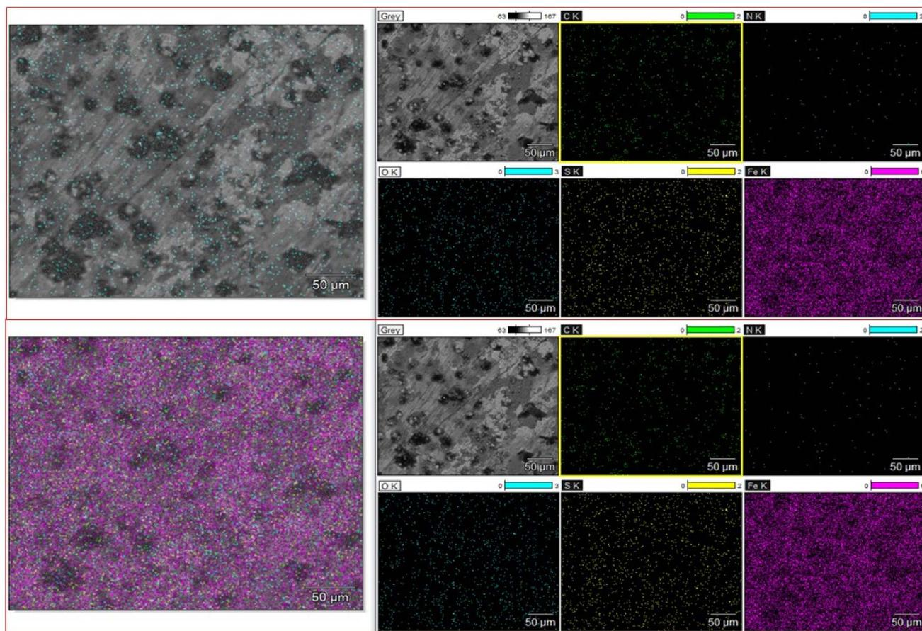
Fig. 10 SEM-EDS mapping of the main element distribution in the carbon steel sample immersed in a 400 ppm HCl-containing CHDEPS3 inhibitor for 24 h.
