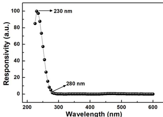
Fig. 8 Normalized spectral selectivity of the Al-doped  $\gamma$ -Ga<sub>2</sub>O<sub>3</sub> thin film-based MSM structure PD.
