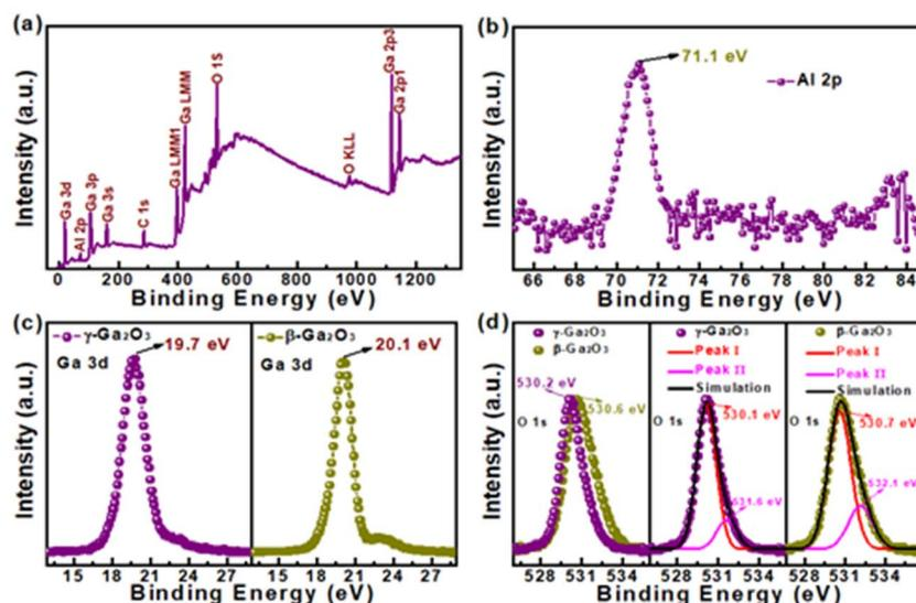
Fig. 4 (a) XPS wide survey spectrum and (b) core level of Al 2p for the Al-doped  $\gamma$ -Ga<sub>2</sub>O<sub>3</sub> film. Core levels of (c) Ga 3d and (d) O 1s for Al-doped  $\gamma$ -Ga<sub>2</sub>O<sub>3</sub> and undoped  $\beta$ -Ga<sub>2</sub>O<sub>3</sub> films.
