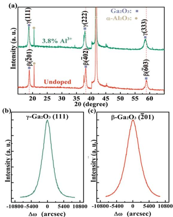
Fig. 2 (a) XRD patterns of undoped and Al-doped  $\text{Ga}_2\text{O}_3$  films. X-ray rocking curves of (b)  $\gamma\text{-Ga}_2\text{O}_3$  (111) for the Al-doped film and (c)  $\beta\text{-Ga}_2\text{O}_3$  (201) for the undoped film.
