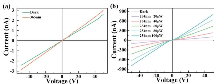
Fig. 5 (a)  $I$ - $V$  characteristics of the Al-doped  $\gamma$ -Ga<sub>2</sub>O<sub>3</sub> thin film-based MSM structure PD in the dark and under a 365 nm light illumination. (b)  $I$ - $V$  characteristics of the device in the dark and under a 254 nm light illumination with various light intensities.
