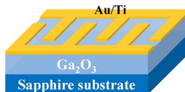
Fig. 1 Schematic of an MSM structure PD.
