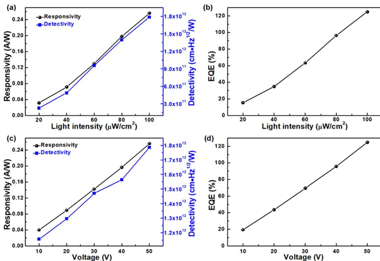
Fig. 7 (a) Responsivity and detectivity of the Al-doped  $\gamma$ -Ga<sub>2</sub>O<sub>3</sub> thin film-based MSM structure PD as a function of bias voltage. (b) External quantum efficiency of the device as a function of bias voltage. (c) Responsivity and detectivity of the device as a function of light intensity. (d) External quantum efficiency of the device as a function of light intensity.
