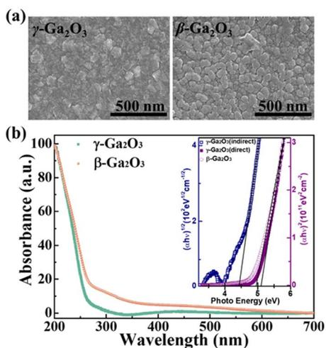
Fig. 3 (a) SEM images of the Al-doped  $\gamma\text{-Ga}_2\text{O}_3$  and undoped  $\beta\text{-Ga}_2\text{O}_3$  films. (b) UV-vis absorbance spectra of the Al-doped  $\gamma\text{-Ga}_2\text{O}_3$  and undoped  $\beta\text{-Ga}_2\text{O}_3$  films with the plot of  $(\alpha h\nu)^2$  and  $(\alpha h\nu)^{1/2}$  vs.  $h\nu$  in the inset.
