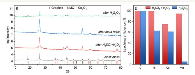
Fig. 4 (a) XRD patterns of a representative probe of black mass and the remaining insoluble fraction after leaching in different etchants; (b) leaching efficiency in  $H_2SO_4 + H_2O_2$  and  $H_2S_2O_8$  etching solutions relative to the aqua regia.
