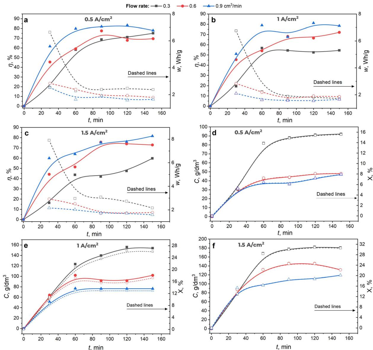
Fig. 2 Dependence of current efficiency and specific energy consumption on time at different flow rates: (a)  $0.5 \text{ A cm}^{-2}$ , (b)  $1 \text{ A cm}^{-2}$ , (c)  $1.5 \text{ A cm}^{-2}$ ; dependence of  $\text{H}_2\text{S}_2\text{O}_8$  concentration and  $\text{H}_2\text{SO}_4$  conversion rate at different flow rates on time: (d)  $0.5 \text{ A cm}^{-2}$ , (e)  $1 \text{ A cm}^{-2}$ , (f)  $1.5 \text{ A cm}^{-2}$ .
