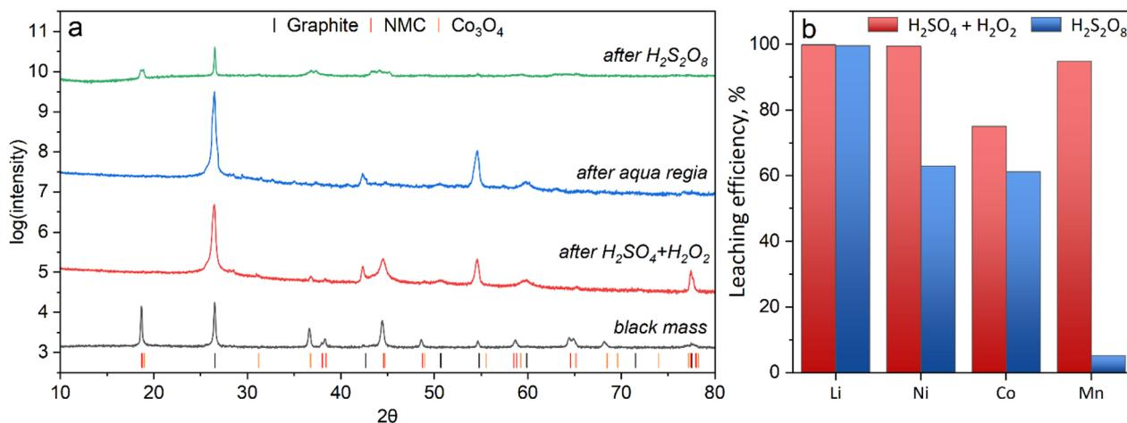
Fig. 4 (a) XRD patterns of a representative probe of black mass and the remaining insoluble fraction after leaching in different etchants; (b) leaching efficiency in  $\text{H}_2\text{SO}_4 + \text{H}_2\text{O}_2$  and  $\text{H}_2\text{S}_2\text{O}_8$  etching solutions relative to the aqua regia.
