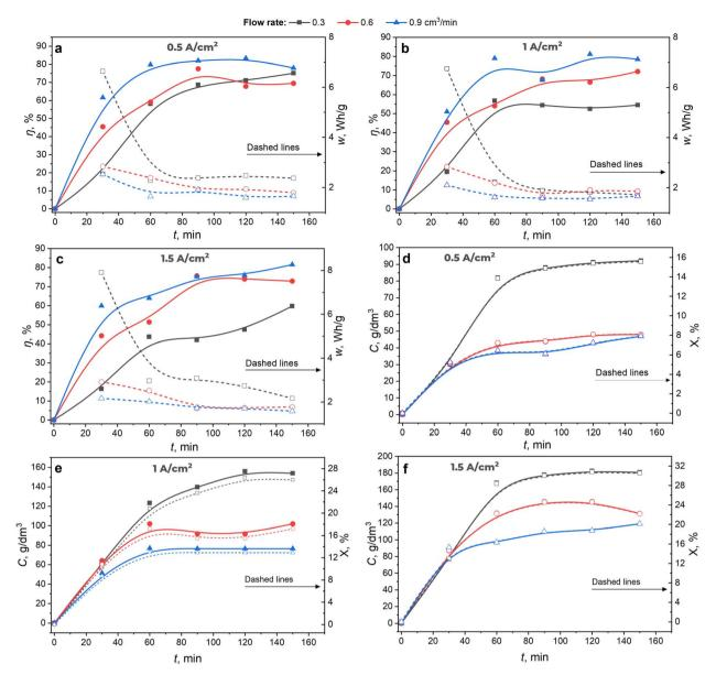
Fig. 2 Dependence of current efficiency and specific energy consumption on time at different flow rates: (a)  $0.5 \,\mathrm{A}\,\mathrm{cm}^{-2}$ , (b)  $1.4 \,\mathrm{cm}^{-2}$ , (c)  $1.5 \,\mathrm{A}\,\mathrm{cm}^{-2}$ ; dependence of  $\mathrm{H}_2\mathrm{S}_2\mathrm{O}_8$  concentration and  $\mathrm{H}_2\mathrm{S}_2\mathrm{O}_8$  conversion rate at different flow rates on time: (d)  $0.5 \,\mathrm{A}\,\mathrm{cm}^{-2}$ , (e)  $1.6 \,\mathrm{A}\,\mathrm{cm}^{-2}$ .
