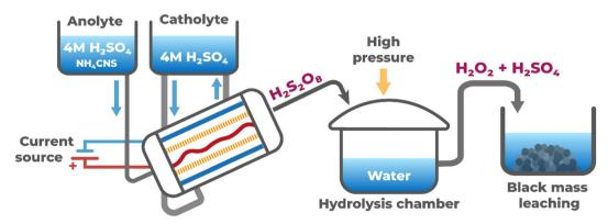
Proposed three-stage industrial process for black mass leaching using electrochemically generated peroxodisulfuric acid.
