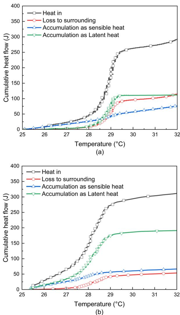
Fig. 9 Cumulative heat flow as a function of paint surface temperature with a PCM loading of  $1.08 \text{ kg m}^{-2}$  for an imposed heat flux of (a)  $62.5 \text{ W m}^{-2}$  and (b)  $350 \text{ W m}^{-2}$ .
