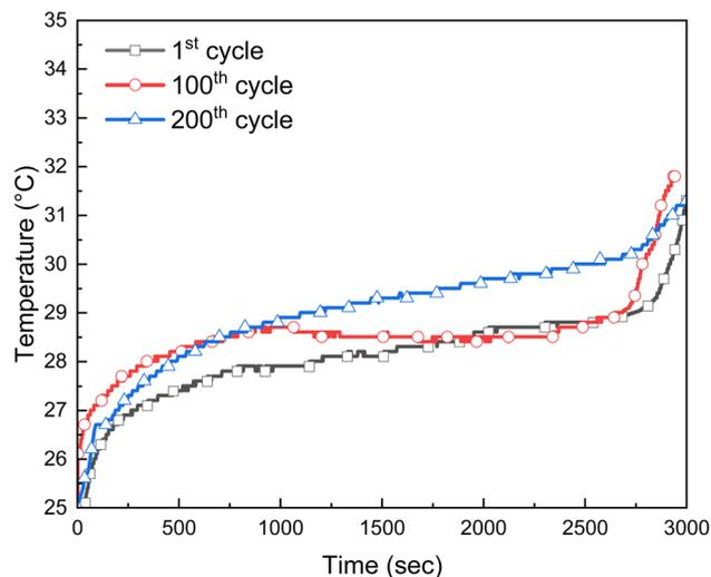
Fig. 11 Temperature profiles of the paint surface at an imposed heat flux of 125 W m<sup>-2</sup> and a PCM loading of 1.08 kg m<sup>-2</sup> after multiple melt-freeze cycles.
