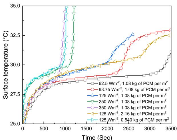
Fig. 6 Build-up of the paint surface temperature at varied heat flux and MPCM loading.
