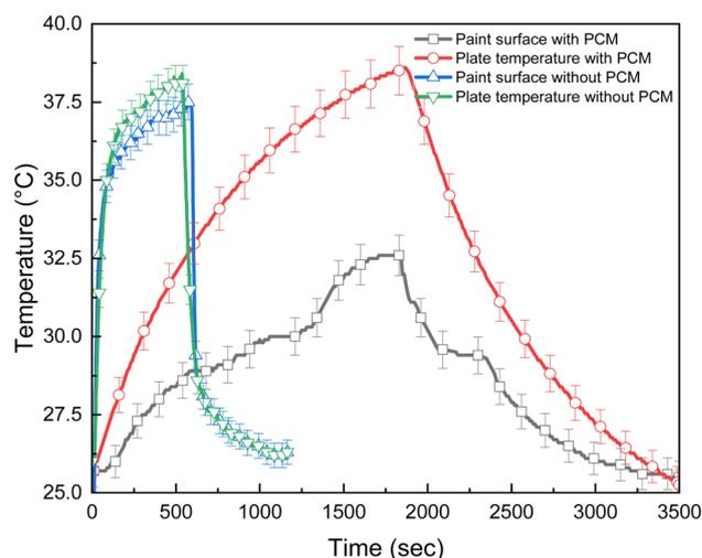
Fig. 5 Build-up of temperature across the aluminium plate at an imposed heat flux of  $125\text{ W m}^{-2}$ .
