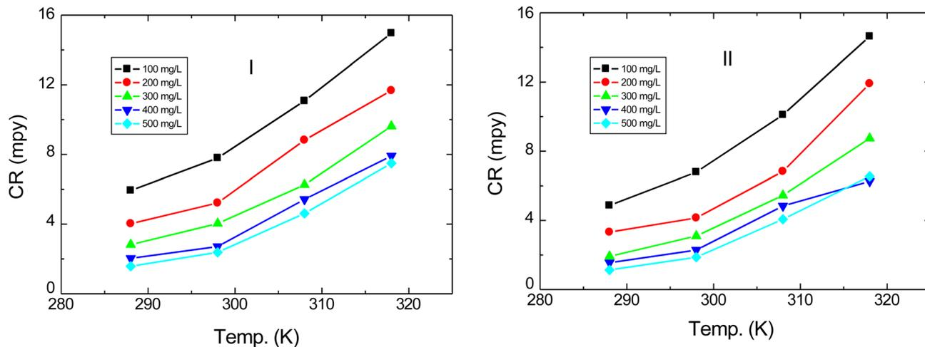
Fig. 8 Variation in the CR of brass in 3.5% NaCl with diverse doses of streptomycin (I) and neomycin (II) with temperature.
