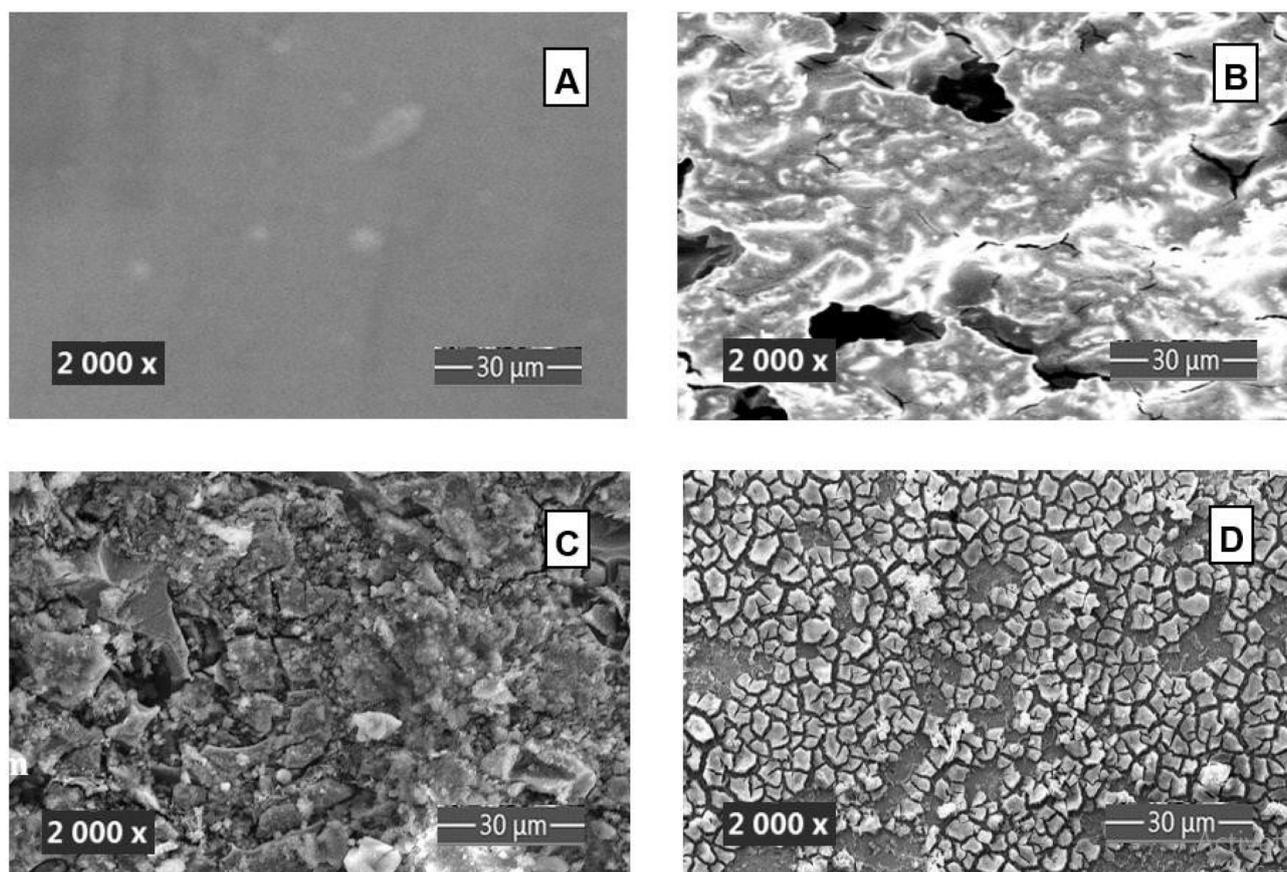
Fig. 18 SEM images (mag. 2000 $\times$ ) of the surfaces of brass (A) before and after 24 hours of immersion in (B) 3.5% NaCl and (C) and (D) 3.5% NaCl with 500 mg L<sup>-1</sup> streptomycin and neomycin, respectively.
