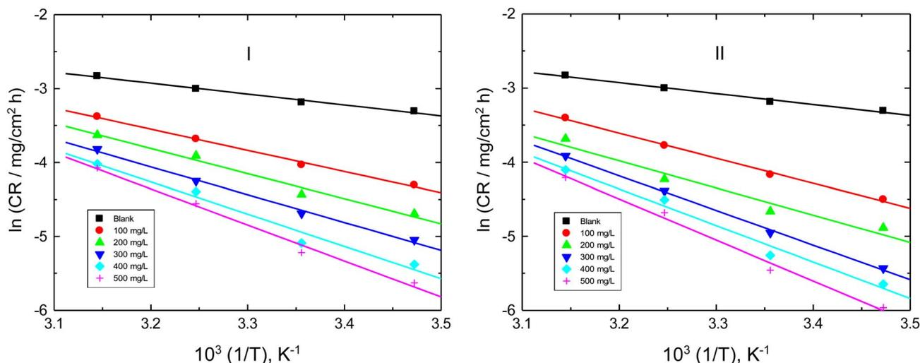
**Fig. 12** Arrhenius plots for the corrosion of brass in 3.5% NaCl with streptomycin (I) and neomycin (II).
