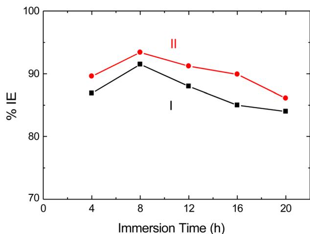
Fig. 7 Variation in the % IEs of streptomycin (I) and neomycin (II) at  $500 \text{ mg L}^{-1}$  with immersion time in the corrosion of brass in 3.5% NaCl at 298 K.
