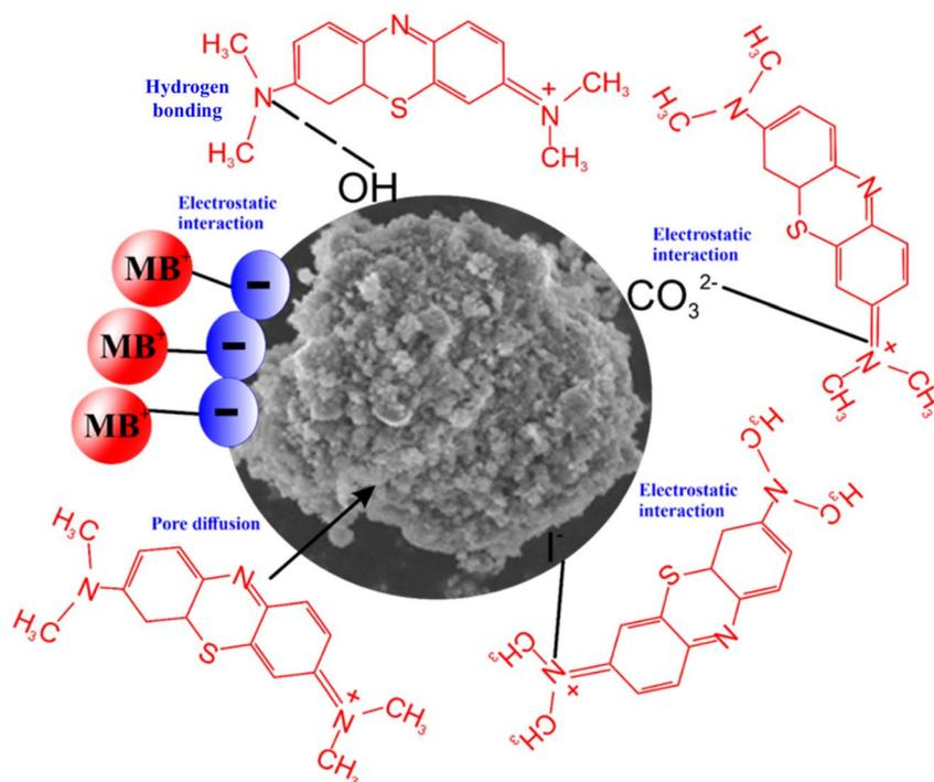
Fig. 8 The possible mechanism for MB adsorption on the RMI-5 surface.
