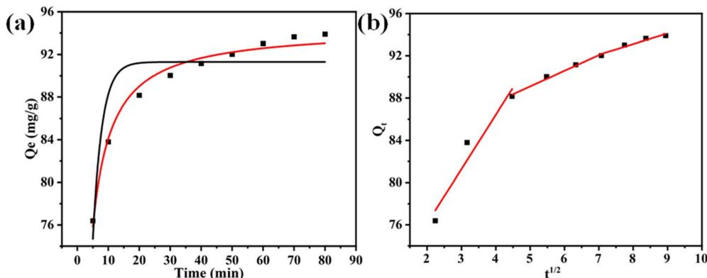
Fig. 6 Kinetic model fit of MB dye: (a) red plot is for PSO and black is for PFO and (b) intraparticle diffusion model.
