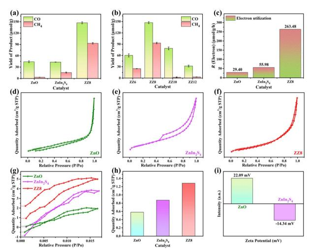
Fig. 4 (a–c)  $CO_2$  photoreduction activity, (d–f)  $N_2$  adsorption–desorption isotherms, (g–h)  $CO_2$  adsorption–desorption isotherms with corresponding net adsorption histogram, and (i) zeta potentials of the samples.
