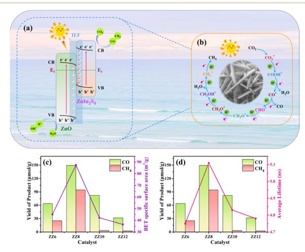
Fig. 9 Schematic diagram for (a) S-scheme charge transfer mechanism and (b) reaction pathway of CO<sub>2</sub> photoreduction over ZnO/ZnIn<sub>2</sub>S<sub>4</sub>; CO<sub>2</sub> photoreduction activity *versus* (c) the BET specific surface area and (d) the average lifetime of photogenerated carriers.
