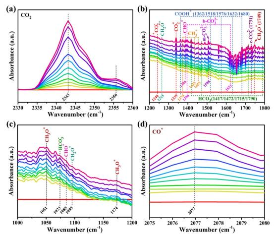
Fig. 8 In situ FTIR spectra of photocatalytic  $CO_2$  reduction over ZZ8 in the regions of (a) 2330-2360 cm<sup>-1</sup>, (b) 1200-1800 cm<sup>-1</sup>, (c) 1000-1200 cm<sup>-1</sup> and (d) 2075-2080 cm<sup>-1</sup>.
