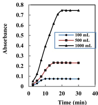
Fig. 3 Effect of shaking time on fixation of complex of 500 ng per mL Zn<sup>2+</sup> for 100, 500 and 1000 mL samples using 65, 50, and 50 mg, respectively, of Dowex1-X8 (400 mesh).
