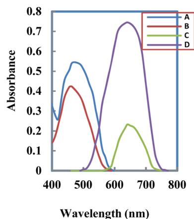
Fig. 1 Absorption spectra of (A) blank in solution (B) blank for SPS, (C) SPS for 500 mL and (D) SPS for 1000 mL samples for 500 ng per mL Zn<sup>2+</sup>.
