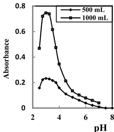
Fig. 2 Effect of pH on fixation and complexation of 500 ng mL<sup>-1</sup> of Zn<sup>2+</sup> ions for 500 and 1000 mL samples using 50 mg of Dowex 400 mesh.
