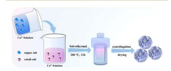
Fig. 1 Schematic diagram of the synthesis of f-CuCo<sub>2</sub>S<sub>4</sub>.
