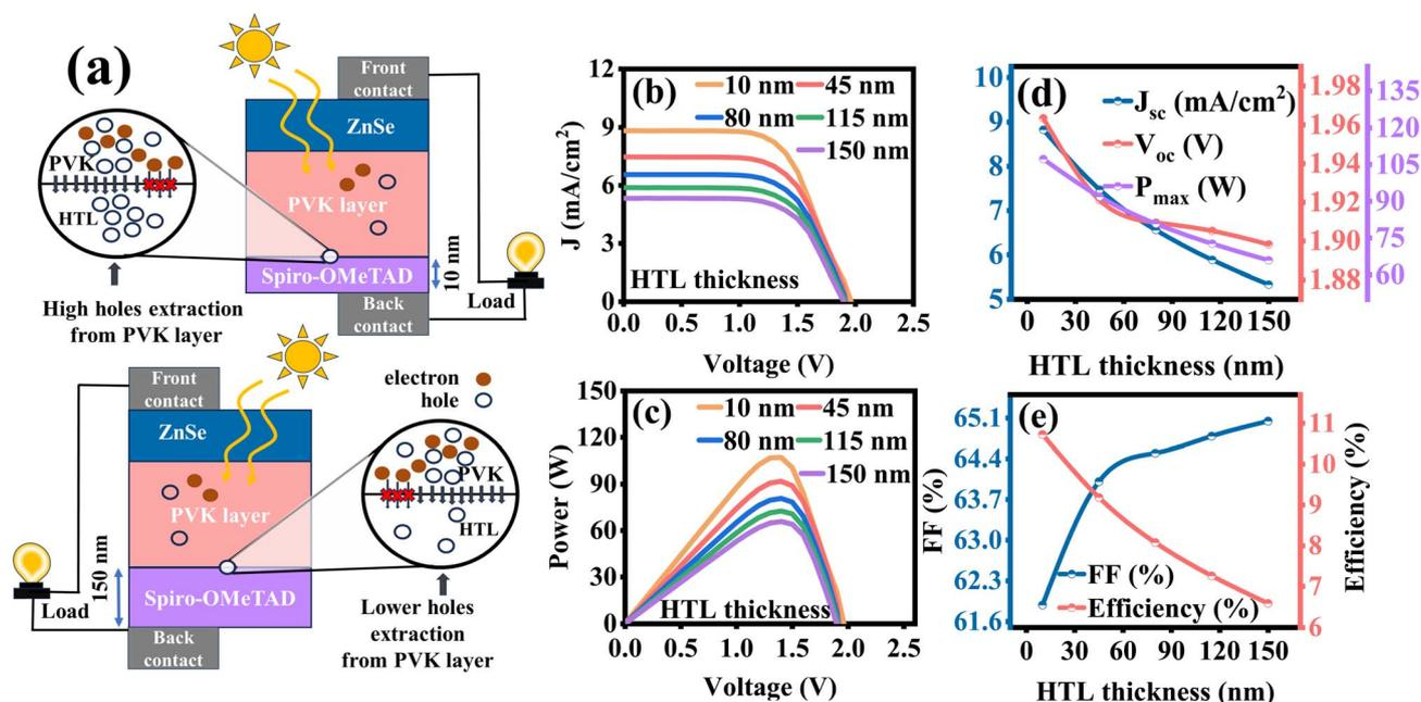
**Fig. 5** (a) Schematic of the solar cell with different absorbing layer thicknesses. (b and c)  $J$ - $V$  &  $P$ - $V$  characteristics, and (d and e) the influence of HTL thickness variation on PV parameters such as  $J_{sc}$ ,  $V_{oc}$ ,  $P_{max}$ , FF, and efficiency.
