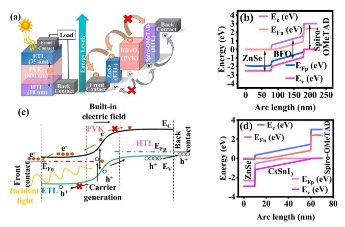
Fig. 2 (a) Structural layout of the proposed solar cell ( $ZnSe/BiFeO_3/spiro-OMeTAD$ ). (b) The energy band diagram of the ZnSe/BFO/spiro-OMeTAD structure, showing alignment across each layer. (c) Visualization of the charge carrier flow and separation within the device. (d) The energy band diagram of the  $ZnSe/CsSnI_3/spiro$  structure, illustrating the band alignment and carrier transport pathways.
