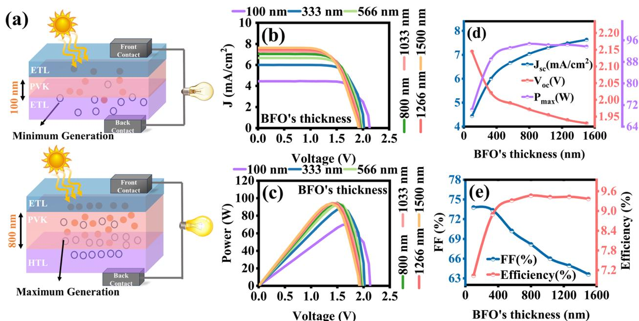
Fig. 3 (a) Schematic showing the comparison between two different thicknesses of the BFO layer in the ZnSe/BiFeO<sub>3</sub>/Spiro-OMeTAD solar cell. (b and c)  $J$ - $V$  &  $P$ - $V$  characteristics, and (d and e) the impact of BFO thickness variation on PV parameters such as  $J_{\text{sc}}$ ,  $V_{\text{oc}}$ ,  $P_{\max}$ , FF, and efficiency.
