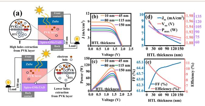
Fig. 5 (a) Schematic of the solar cell with different absorbing layer thicknesses. (b and c) J-V + P-V characteristics, and (d and e) the influence of HTL thickness variation on PV parameters such as  $J_{sc}$ ,  $V_{oc}$ ,  $P_{max}$ , FF, and efficiency.
