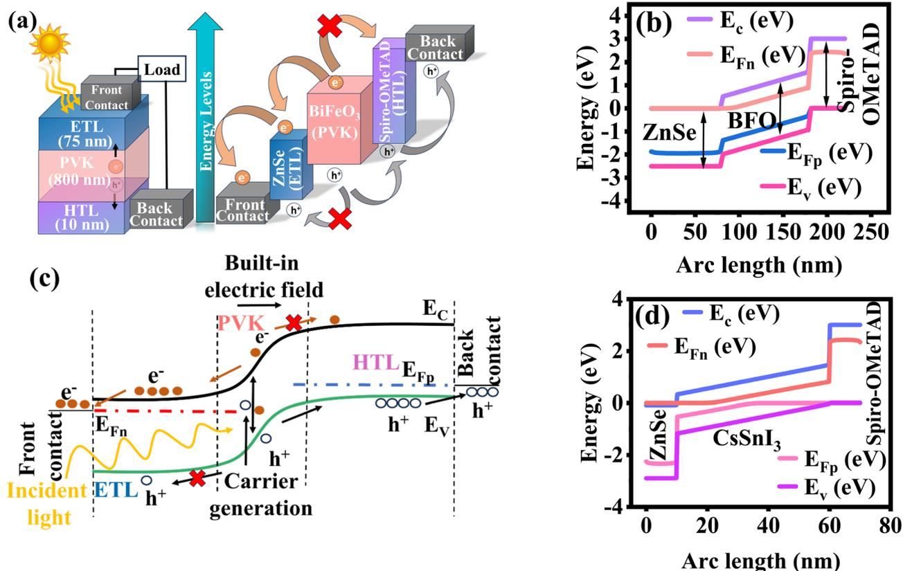
Fig. 2 (a) Structural layout of the proposed solar cell (ZnSe/BiFeO<sub>3</sub>/spiro-OMeTAD). (b) The energy band diagram of the ZnSe/BFO/spiro-OMeTAD structure, showing alignment across each layer. (c) Visualization of the charge carrier flow and separation within the device. (d) The energy band diagram of the ZnSe/CsSnI<sub>3</sub>/spiro structure, illustrating the band alignment and carrier transport pathways.
