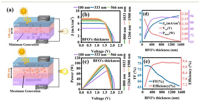
Fig. 3 (a) Schematic showing the comparison between two different thicknesses of the BFO layer in the ZnSe/BiFeO<sub>3</sub>/spiro-OMeTAD solar cell. (b and c)  $J-V\otimes P-V$  characteristics, and (d and e) the impact of BFO thickness variation on PV parameters such as  $J_{sc}$ ,  $V_{oc}$ ,  $P_{max}$ , FF, and efficiency.
