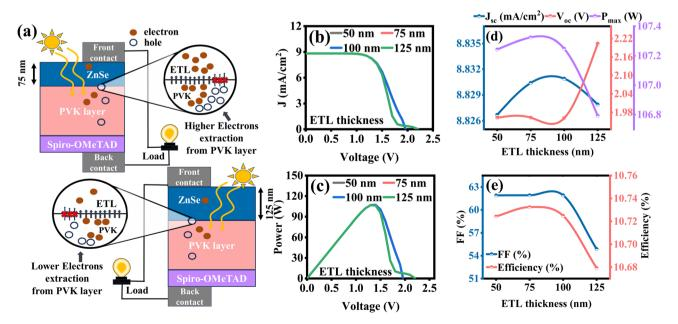
Fig. 4 (a) Schematic visualization of the ZnSe/BiFeO<sub>3</sub>/spiro-OMeTAD solar cell with varied ETL thicknesses. (b and c) J-V & P-V characteristics, and (d and e) the effect of the ETL thickness variation on PV parameters such as  $J_{\text{sc}}$ ,  $V_{\text{oc}}$ ,  $P_{\text{max}}$ , FF, and efficiency.
