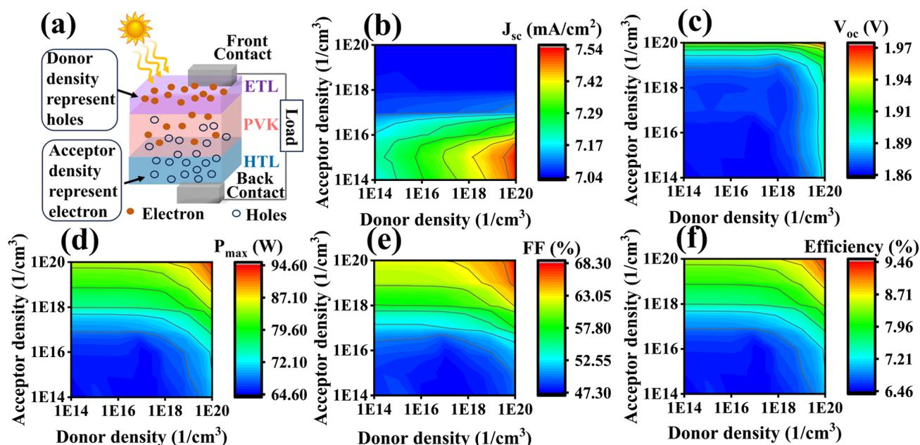
Fig. 6 (a) Schematic depiction of donor and acceptor concentrations, highlighting their role in performance; (b–f) corresponding trends in PV performance metrics with varying carrier densities, such as  $J_{sc}$ ,  $V_{oc}$ ,  $P_{max}$ , FF, and efficiency, respectively.
