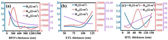
Fig. 7 Variation in series resistance ( $R_s$ ), shunt resistance ( $R_{sh}$ ), and characteristic resistance ( $R_{ch}$ ) with respect to the (a) absorbing layer (BFO) thickness, (b) ETL thickness, and (c) HTL thickness.
