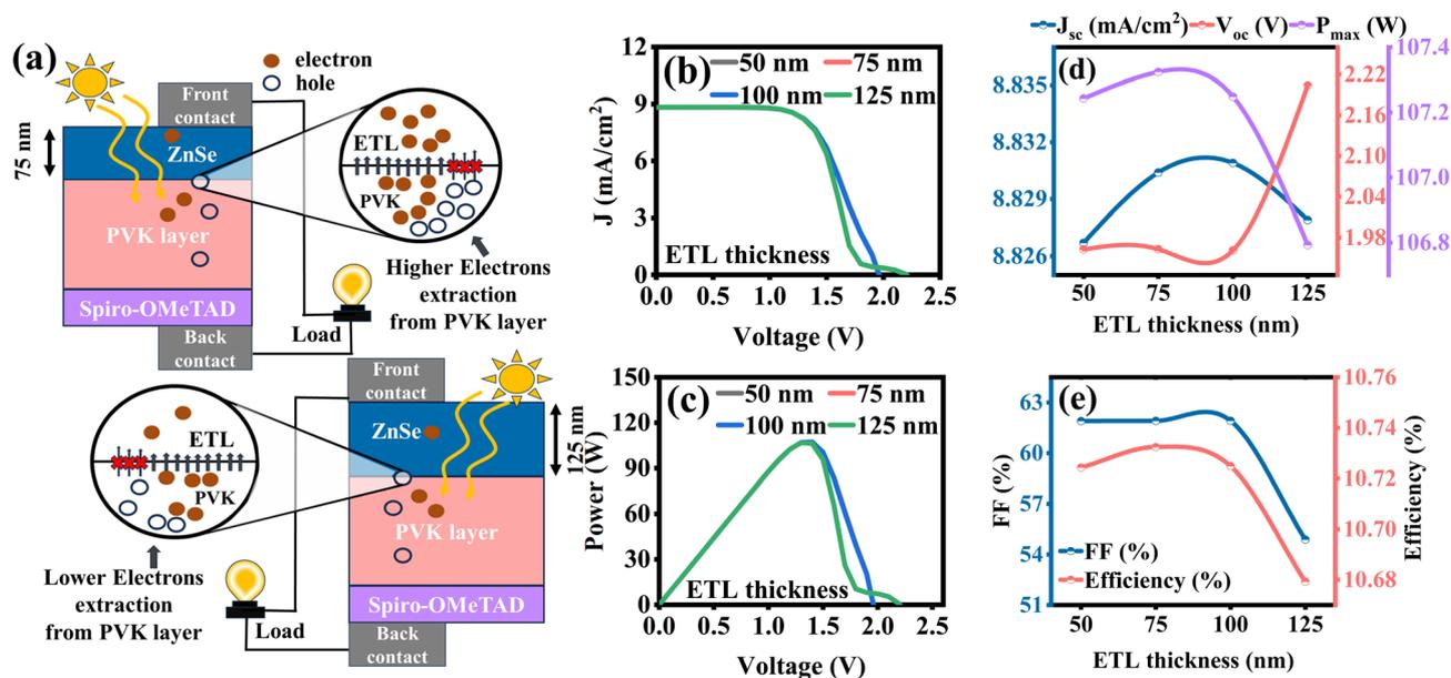
**Fig. 4** (a) Schematic visualization of the ZnSe/BiFeO<sub>3</sub>/spiro-OMeTAD solar cell with varied ETL thicknesses. (b and c)  $J$ - $V$  &  $P$ - $V$  characteristics, and (d and e) the effect of the ETL thickness variation on PV parameters such as  $J_{sc}$ ,  $V_{oc}$ ,  $P_{max}$ , FF, and efficiency.
