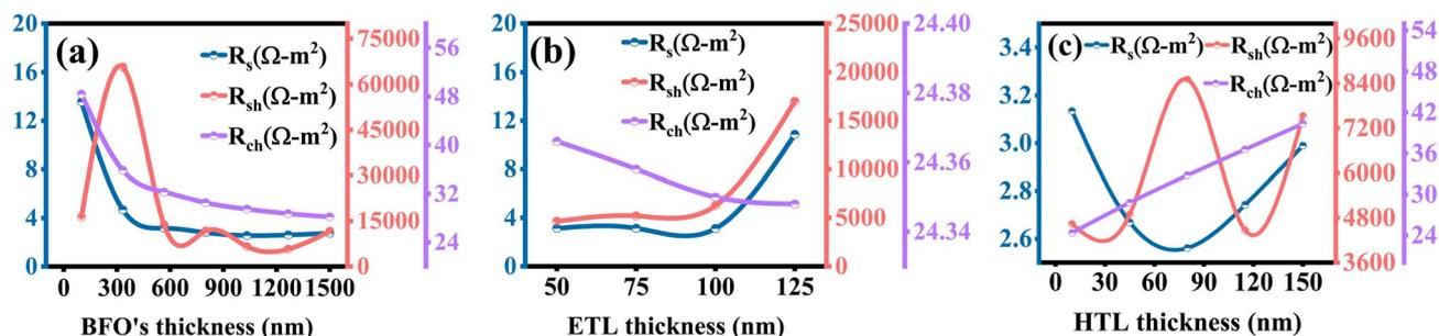
Fig. 7 Variation in series resistance ( $R_s$ ), shunt resistance ( $R_{sh}$ ), and characteristic resistance ( $R_{ch}$ ) with respect to the (a) absorbing layer (BFO) thickness, (b) ETL thickness, and (c) HTL thickness.
