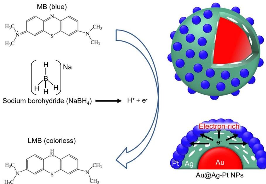
Fig. 9 The schematic diagram of the probable MB reduction mechanism in the presence of the Au@Ag–Pt NPs and NaBH<sub>4</sub>.
