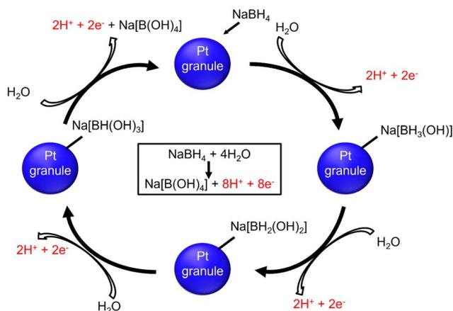
Fig. 10 Mechanism of the hydrolysis of sodium borohydride as catalyzed by the surficial Pt granule.
