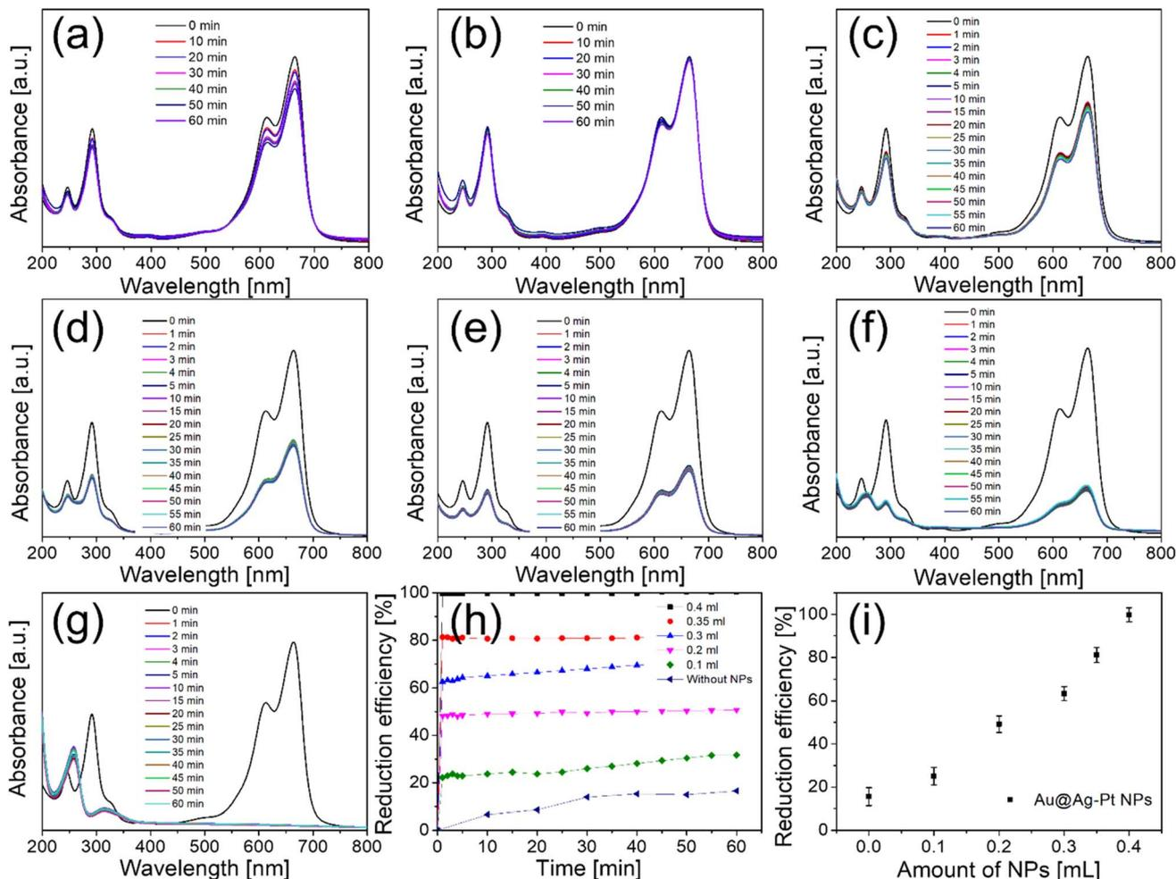
Fig. 5 The UV-vis absorption spectra illustrating the reduction of MB dye under different conditions: (a) without Au@Ag-Pt NPs, (b) without  $\text{NaBH}_4$  but with varying volumes of Au@Ag-Pt NPs: (c) 0.10 mL, (d) 0.20 mL, (e) 0.30 mL, (f) 0.35 mL, (g) 0.40 mL, and (h and i) the corresponding reduction efficiency after 60 minutes.
