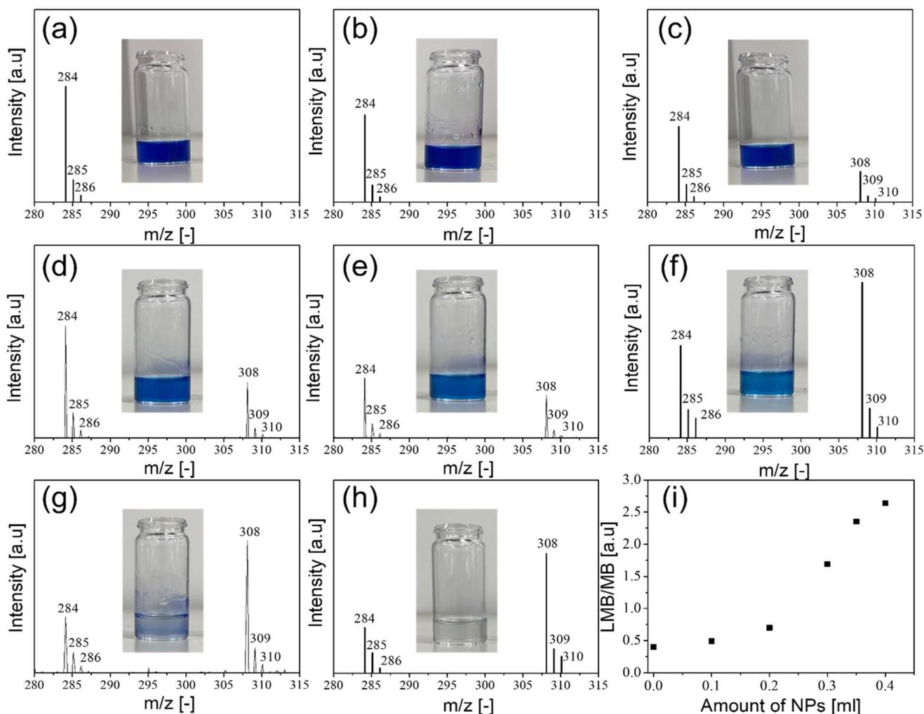
Fig. 7 The ESI-MS in the positive mode for (a) pure MB, (b) pure MB with NPs (0.4 mL), (c) pure MB with  $\text{NaBH}_4$ , and pure MB containing  $\text{NaBH}_4$  with various amounts of Au@Ag–Pt NPs: (d) 0.10 mL, (e) 0.20 mL, (f) 0.30 mL, (g) 0.35 mL, (h) 0.40 mL. (i) Is the  $m/z$  ratio of LMB/MB measured for various amounts of Au@Ag–Pt NPs. The inset images show the gradual color changes from the MB to the reduced MB (LMB) due to the reduction of MB, as seen in (i).
