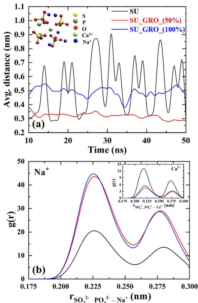
Fig. 3 (a) Ion complexation among  $\text{PO}_4^{3-}$  and  $\text{SO}_4^{2-}$  mediated by  $\text{Ca}^{2+}$  and  $\text{Na}^+$  counterions of synthetic urine (SU); (b) radial number density distribution of  $\text{Na}^+$  and  $\text{Ca}^{2+}$  (inset figure) ions in between the  $\text{PO}_4^{3-}$  and  $\text{SO}_4^{2-}$  complexes.
