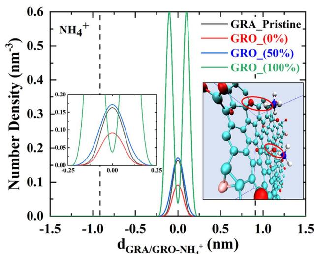
Fig. 5 Snapshot of MD simulation showing the interaction of  $\text{NH}_4^+$  with the deprotonated hydroxyl groups of GRO (100%). Linear density distribution of the  $\text{NH}_4^+$  ion representing its interaction with the interface of GRA/GRO at different conditions considered in this study. GRA (unfunctionalized graphene), GRO (functionalized graphene) and % (percentage of charge on surface).
