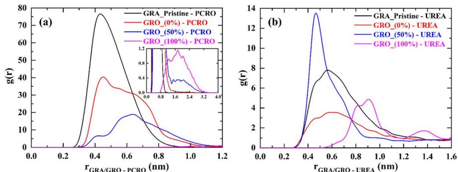
Fig. 8 (a) p-cresol and (b) urea interactions with GRA/GRO sheets in synthetic. GRA (unfunctionalized graphene), GRO (functionalized graphene), % (percentage of charge on surface) and PCRO (p-cresol).
