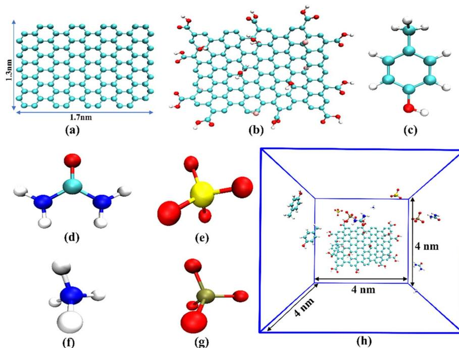
Fig. 1 Snapshots representing the major constituents of simulation box (a) graphene; (b) graphene oxide; (c) p-cresol; (d) urea; (e) sulphate; (f) ammonium; (g) phosphate; (h) representative unit cell of the simulation, all the water molecules were removed for visual clarity.
