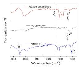
Fig. 3 FTIR spectra of Fe<sub>3</sub>O<sub>4</sub>@SiO<sub>2</sub> NPs, amino modified aptamer (8.28A), and Aptamer-Fe<sub>3</sub>O<sub>4</sub>@SiO<sub>2</sub> NPs.
