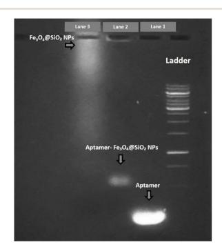
Fig. 4 Gel electrophoresis applied to investigate the bioconjugation of Aptamer to  $Fe_3O_4$  @SiO<sub>2</sub> NPs. Lane 1: Aptamer; Lane 2: Aptamer- $Fe_3O_4$ @SiO<sub>2</sub> NPs; Lane 3,  $Fe_3O_4$ @SiO<sub>2</sub> NPs.
