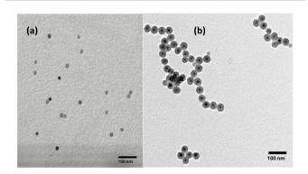
Fig. 1 (a) TEM micrographs of (a) Fe<sub>3</sub>O<sub>4</sub> NPs, (b) Fe<sub>3</sub>O<sub>4</sub>@SiO<sub>2</sub> NPs.
