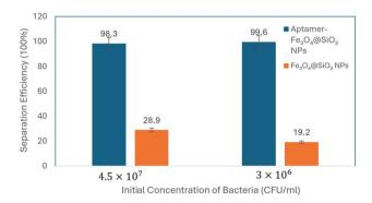
Fig. 8 Living E. coli DH5 $\alpha$  after 10 minutes of magnetic separation with aptamer-MNPs and MNPs at 0.1 $\times$  and 0.01 $\times$  dilutions. The control is core–shell MNPs without aptamer. Bars represent the mean of four replicates.
