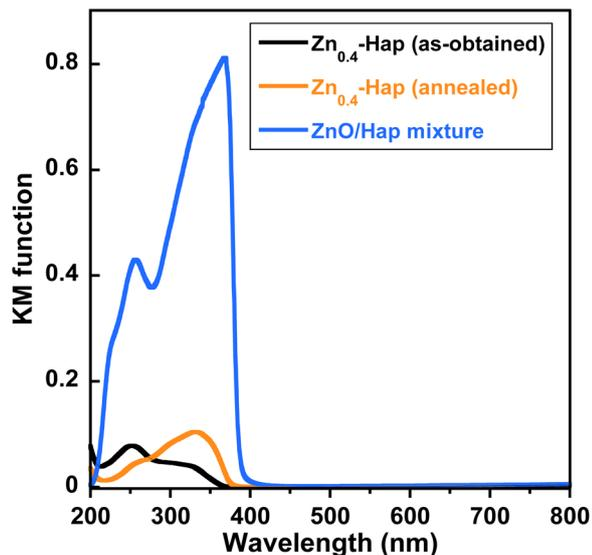
Fig. 10 UV-vis DR spectra of  $\text{Zn}_{0.4}\text{-Hap}$  before and after annealing at  $700\text{ }^\circ\text{C}$ , and the ZnO/Hap mixture. The ZnO/Hap mixing ratio was fixed assuming that all the Zn was deposited from  $\text{Zn}_{0.4}\text{-Hap}$ .
