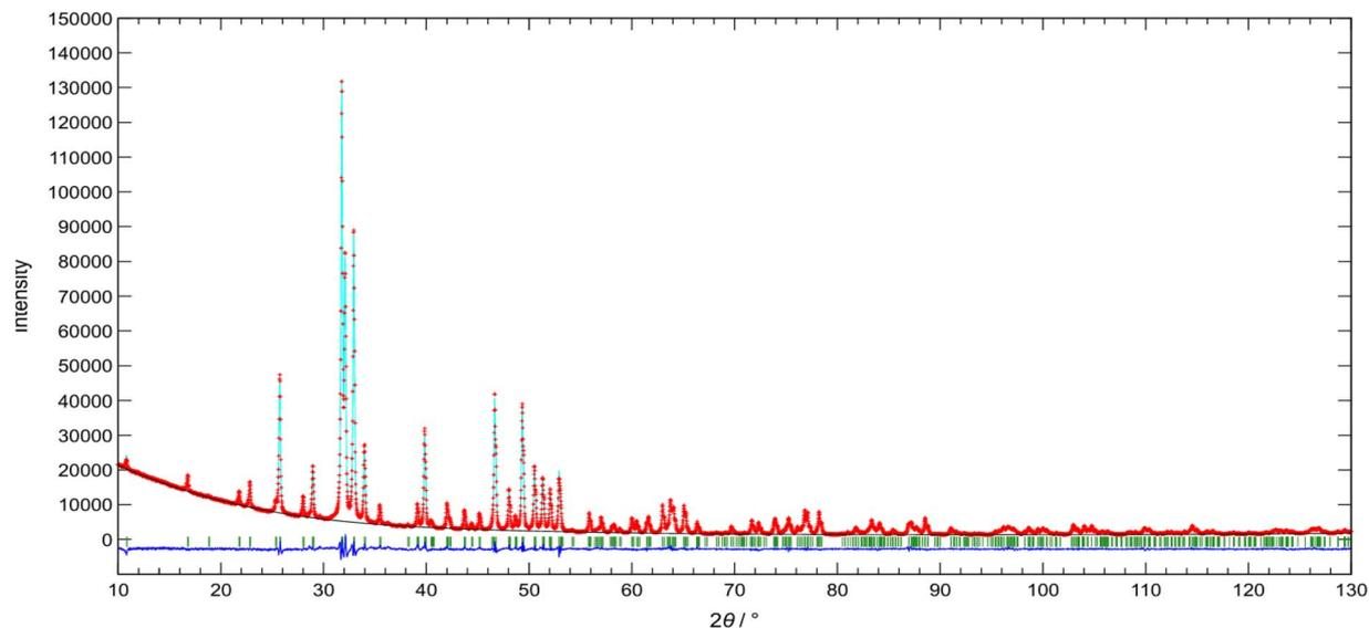
Fig. 4 XRD pattern of  $\text{Zn}_{0.4}\text{-Hap}$ ; experimental (crosses) and calculated (solid line) curves of the Rietveld refinement. The bottom lines show the difference between the two curves. The positions of the apatite phase are shown as vertical lines.
