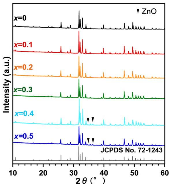
Fig. 1 XRD patterns of  $Zn_x$ -Hap (wet).
