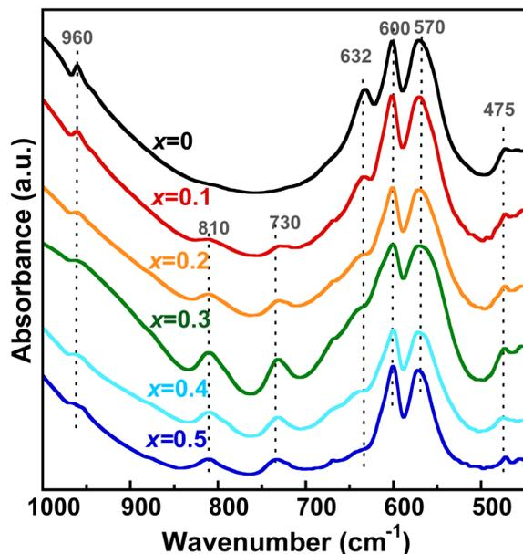
Fig. 6 IR spectra of  $Zn_x$ -Hap.
