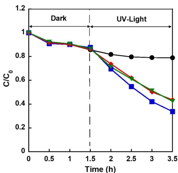
Fig. 12 Changes in the  $C/C_0$  of MB in the presence of  $Zn_{0.4}$ -Hap (as-obtained) (black),  $Zn_{0.4}$ -Hap annealed for 3 h (blue) or 9 h (red) and ZnO@Hap (green) under dark and light irradiation.
