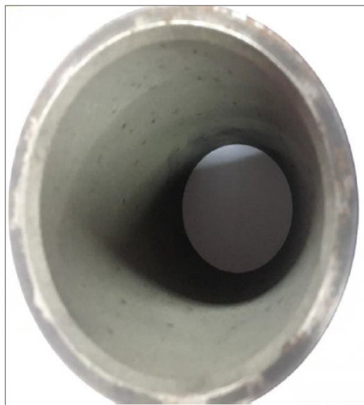
Fig. 3 Fly ash powder-coated cylinder liner.
