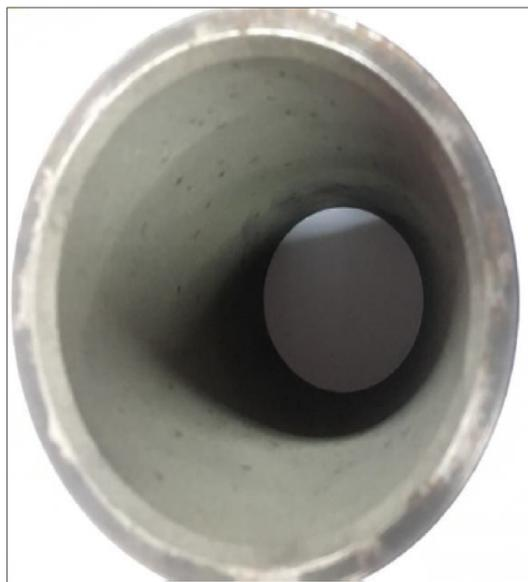
Fig. 3 Fly ash powder-coated cylinder liner.
