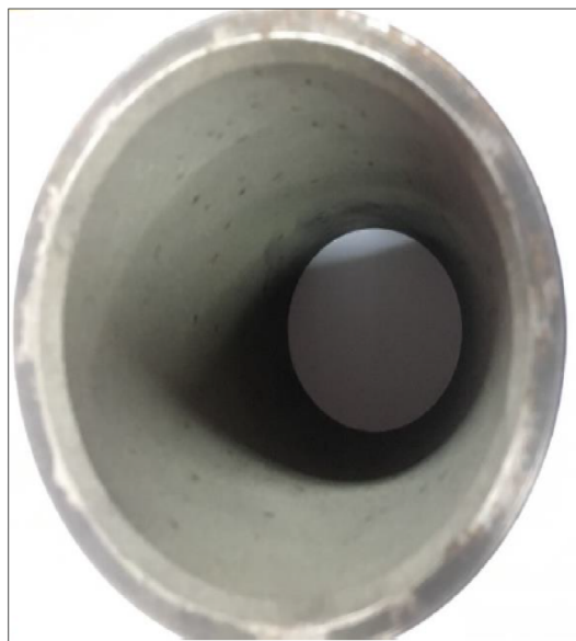
Fig. 3 Fly ash powder-coated cylinder liner.
