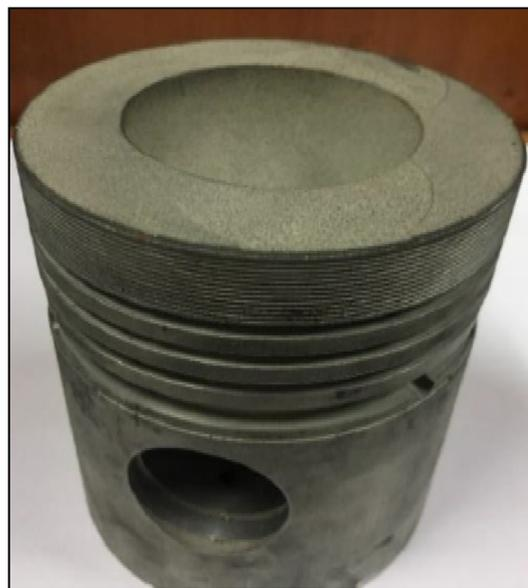
Fig. 2 Fly ash powder-coated piston crown.
