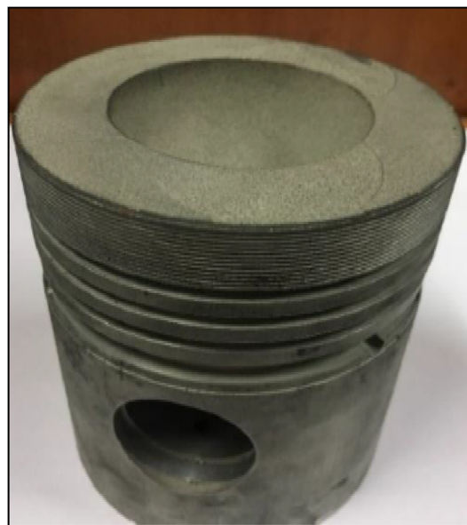
Fig. 2 Fly ash powder-coated piston crown.
