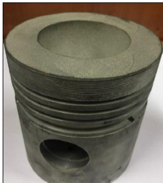
Fig. 2 Fly ash powder-coated piston crown.
