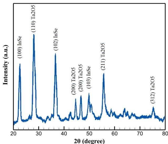
Fig. 2 XRD pattern of the InSe QD/Ta<sub>2</sub>O<sub>5</sub> nanocomposite recorded using Cu K $\alpha$  radiation ( $\lambda = 1.5406$   $\text{\AA}$ ).
