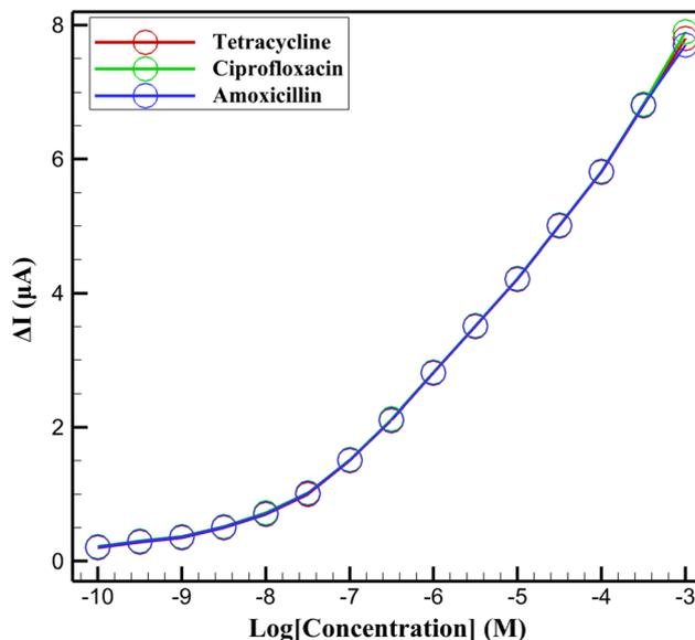
Fig. 11 DPV calibration curves ( $\Delta I$  vs.  $\log[\text{concentration}]$ ) for tetracycline (red solid), ciprofloxacin (green solid), and amoxicillin (blue solid) using InSe QD/Ta<sub>2</sub>O<sub>5</sub>/GCE in 0.1 M PBS with 5 mM K<sub>3</sub>[Fe(CN)<sub>6</sub>]/K<sub>4</sub>[Fe(CN)<sub>6</sub>].
