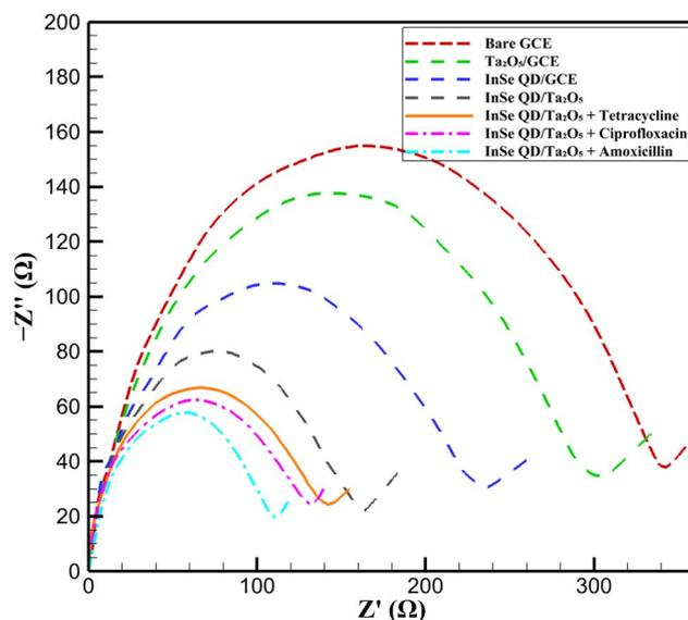
Fig. 8 Nyquist plots of bare GCE, Ta<sub>2</sub>O<sub>5</sub>/GCE, InSe QD/GCE, and InSe QD/Ta<sub>2</sub>O<sub>5</sub>/GCE, with/without 10 µM antibiotics, in 0.05 M PBS (pH 7.4) with 5 mM [Fe(CN)<sub>6</sub>]<sup>3−/4−</sup>.
