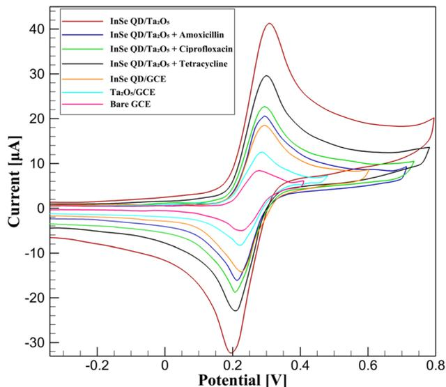
Fig. 7 Cyclic voltammograms of bare GCE, Ta<sub>2</sub>O<sub>5</sub>/GCE, InSe QD/GCE, and InSe QD/Ta<sub>2</sub>O<sub>5</sub>/GCE, with and without 10 µM tetracycline, ciprofloxacin, and amoxicillin, in 0.1 M PBS (pH 7.4) with 5 mM [Fe(CN)<sub>6</sub>]<sup>3−/4−</sup> at 50 mV s<sup>−1</sup>.
