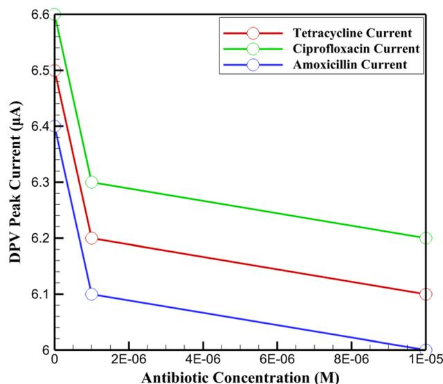
Fig. 14 DPV peak currents of the InSe QD/Ta<sub>2</sub>O<sub>5</sub>-modified GCE for tetracycline, ciprofloxacin, and amoxicillin at concentrations of 10<sup>-6</sup> M and 10<sup>-5</sup> M in simulated river water (0.1 M PBS with 0.5 mg per mL humic acid), measured in 0.1 M PBS (pH 7.4) with 5 mM K<sub>3</sub>[Fe(CN)<sub>6</sub>]/K<sub>4</sub>[Fe(CN)<sub>6</sub>].
