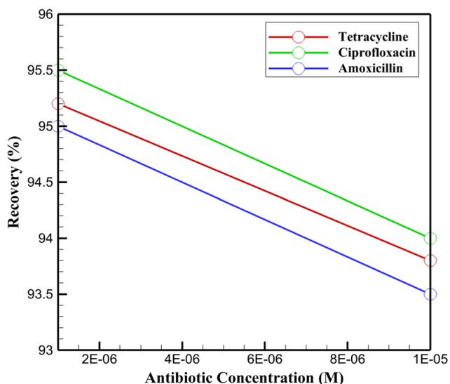
Fig. 13 Recovery percentages of the InSe QD/Ta<sub>2</sub>O<sub>5</sub>-modified GCE for tetracycline, ciprofloxacin, and amoxicillin at concentrations of 10<sup>-6</sup> M and 10<sup>-5</sup> M in simulated river water (0.1 M PBS with 0.5 mg mL<sup>-1</sup> humic acid), measured *via* DPV in 0.1 M PBS (pH 7.4) with 5 mM K<sub>3</sub>[Fe(CN)<sub>6</sub>]/K<sub>4</sub>[Fe(CN)<sub>6</sub>].
