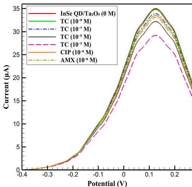
Fig. 15 CV of InSe QD/Ta<sub>2</sub>O<sub>5</sub>-modified GCE in 0.1 M PBS (pH 7.4) with 5 mM K<sub>3</sub>[Fe(CN)<sub>6</sub>]/K<sub>4</sub>[Fe(CN)<sub>6</sub>], showing baseline (0 M, red line) and responses to tetracycline (TC) at 10<sup>-9</sup> to 10<sup>-3</sup> M, ciprofloxacin (CIP) at 10<sup>-6</sup> M, and amoxicillin (AMX) at 10<sup>-6</sup> M.
