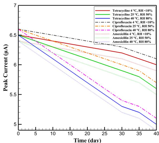
Fig. 12 Long-term stability of the InSe QD/Ta<sub>2</sub>O<sub>5</sub>-modified GCE for  $10^{-6}$  M tetracycline, ciprofloxacin, and amoxicillin under storage conditions of 4 °C (RH  $<10\%$ ), 25 °C (RH 50%), and 40 °C (RH 80%) over 40 days, measured via DPV in 0.1 M PBS (pH 7.4) with 5 mM K<sub>3</sub>[Fe(CN)<sub>6</sub>]/K<sub>4</sub>[Fe(CN)<sub>6</sub>].
