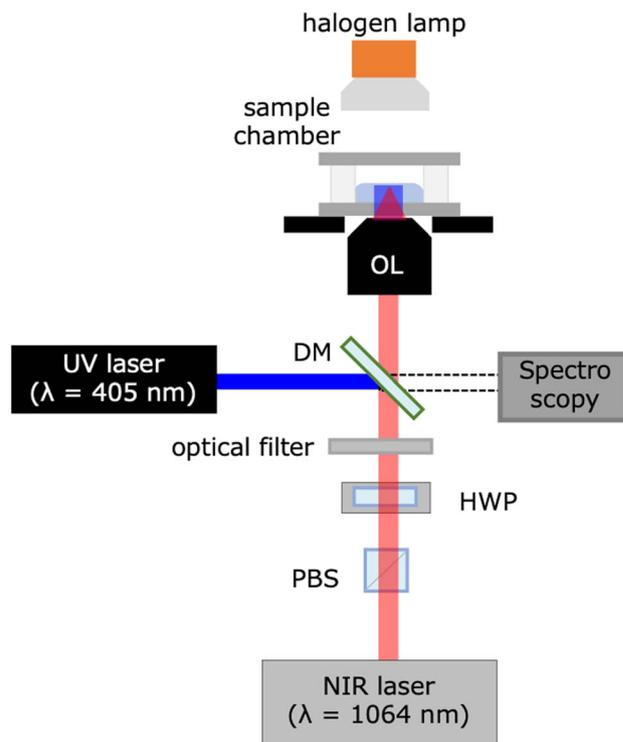
Fig. 2 Optical setup for laser-trapping halide exchange (MAPbBr<sub>3</sub> + MAI → MAPb(Br<sub>1-x</sub>I<sub>x</sub>)<sub>3</sub>) to determine reaction kinetics. A 1064 nm (0.5 W) Nd:YAG laser serves as the trapping source, and a 405 nm (4 mW) laser was used for emission imaging. PBS = polarizing beam splitter; HW = half-wave plate; DM = dichroic mirror.
