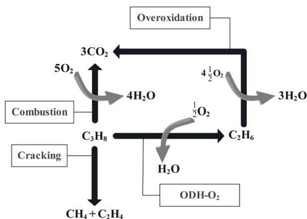
Fig. 2 Typical reaction routes seen in ODH-O<sub>2</sub> reactions. In addition to ODH-O<sub>2</sub>, combustion, overoxidation, and cracking also occur. Adapted from ref. 3 with permission from the Royal Society of Chemistry, copyright 2021 (open access article under CC BY 3.0).
