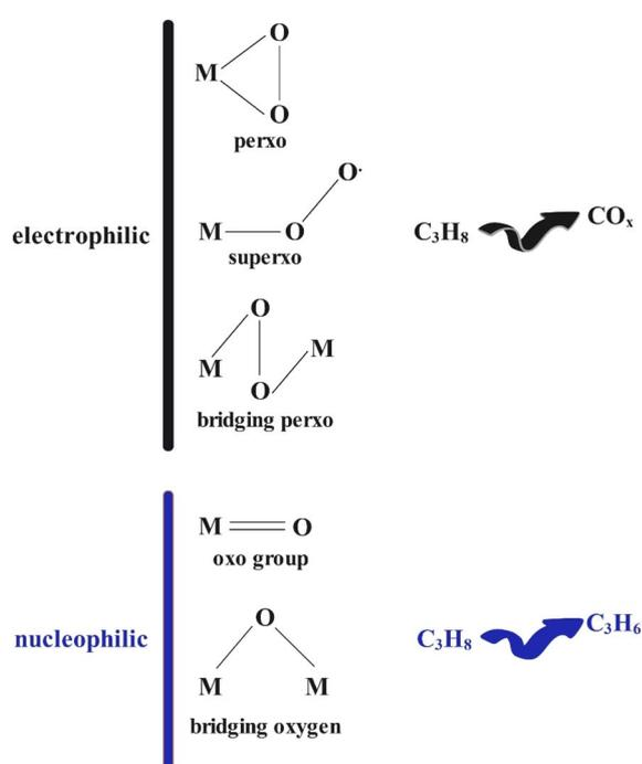
Fig. 3 Diagram illustration of oxygen compounds on catalysts made from metal oxides.
