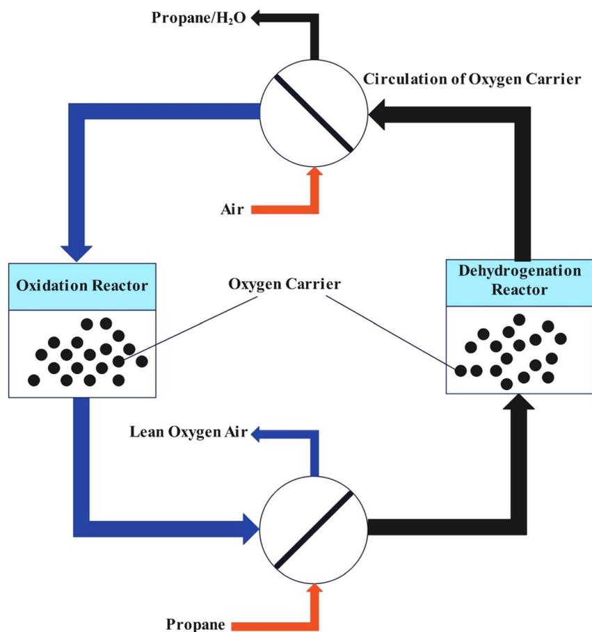
Fig. 4 Schematic of chemical looping ODHP, showing propane feed into the reduction reactor, propylene and by-products exiting to separation, oxygen-depleted carrier transfer to the oxidation reactor, re-oxidation with air, and return of the regenerated carrier. Heat exchange between reactors supports endothermic dehydrogenation.
