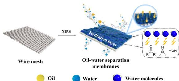
Fig. 8 Schematic illustration of the underwater self-cleaning mechanism of the separation membrane. The underwater oil repellency was on account of the formation of the hydration layer.
