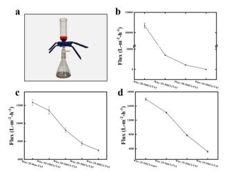
Fig. 5 (a) The image of the testing device. Water fluxes of the prepared wire mesh-based oil–water separation membranes with the varied concentrations of (b) PVDF, (c)  $SbCl_3$ , and (d) TA.
