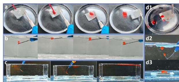
Fig. 7 (a–c) Self-cleaning behavior of the wire/25-3 $\text{SbCl}_3$ /TA3 membrane. (d1–d3) The comparison oil resistance of wire/25–raw/water membrane. (a, d1) The membrane was cut into 2 cm  $\times$  2 cm pieces and then thoroughly rinsed with deionized water before tests. (b, c, d2, d3) The membrane was cut into small pieces measuring approximately 2 cm  $\times$  2 cm and affixed to a slide using double-sided adhesive. Oil was dyed with Sudan red for better observation.
