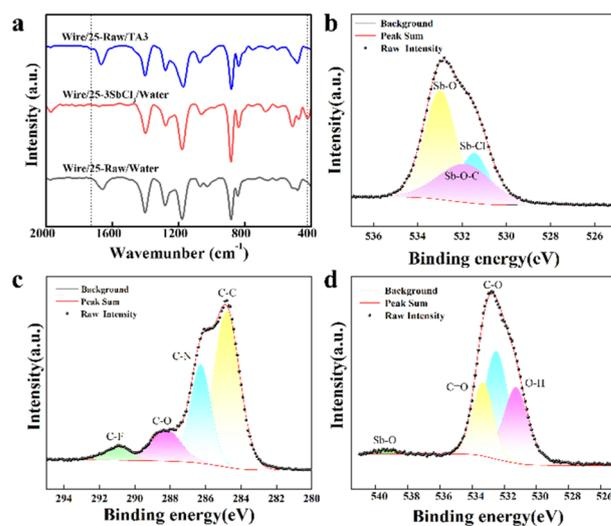
Fig. 4 (a) FTIR spectra of the wire mesh-based oil–water separation membranes. The (b)  $\text{Sb}_{3d}$ , (c) C1s, and (d) O1s peaks of XPS spectra of the wire/25-3 $\text{SbCl}_3$ /TA3 membrane surfaces.
