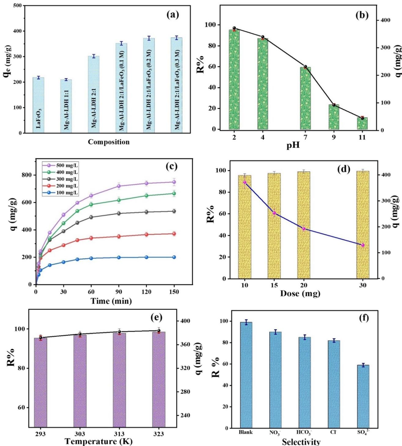
Fig. 4 Optimization of phosphate adsorption on the MgAl-LDH/LaFeO<sub>3</sub> composite: (a) composite composition, (b) pH, (c) initial P-ion concentration, (d) dose, (e) temperature, and (f) selectivity.
