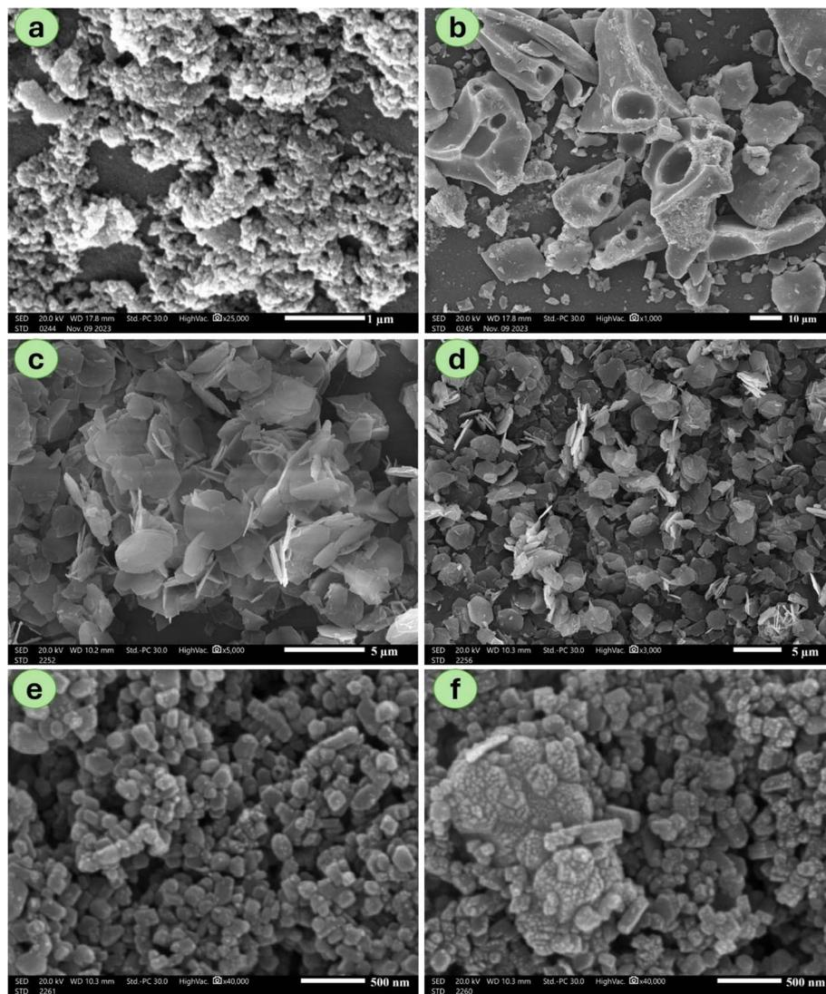
Fig. 2 SEM images of LaFeO<sub>3</sub> (a and b), MgAl-LDH and (c and d) and the MgAl-LDH/LaFeO<sub>3</sub> composite (e and f).
