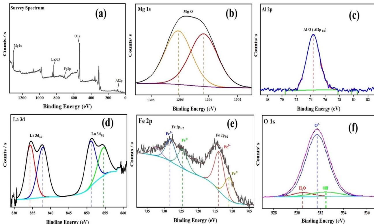
Fig. 3 XPS spectra of the MgAl-LDH/LaFeO<sub>3</sub> composite: (a) survey-spectrum and (b) Mg 1s, (c) Al 2p, (d) La 3d, (e) Fe 2p, and (f) O 1s spectra.
