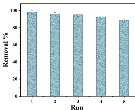
Fig. 9 Reusability of the MgAl-LDH/LaFeO<sub>3</sub> composite for the removal of P-ions.
