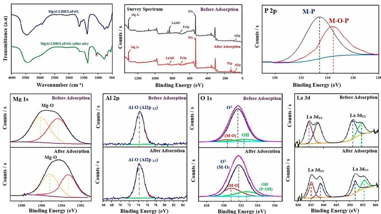
Fig. 7 Characterization of the used MgAl-LDH/LaFeO<sub>3</sub> composite. (a) FTIR, (b) XPS survey, (c) P 2p spectra, (d) Mg 1s spectra, (e) Al 2p spectra, (f) O 1s spectra, and (g) La 3d spectra.
