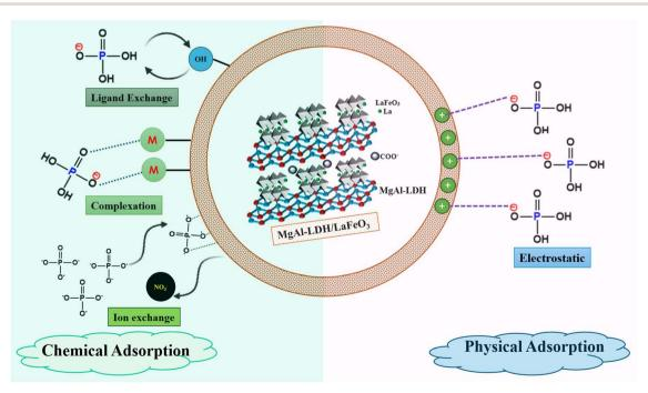
Fig. 8 Adsorption mechanism of P-ions by the MgAl-LDH/LaFeO<sub>3</sub> composite.
