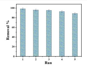
Fig. 9 Reusability of the MgAl-LDH/LaFeO<sub>3</sub> composite for the removal of P-ions.
