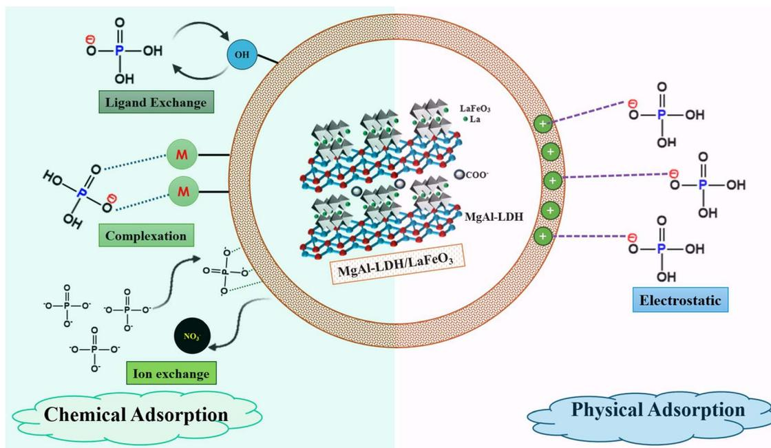
Fig. 8 Adsorption mechanism of P-ions by the MgAl-LDH/LaFeO<sub>3</sub> composite.
