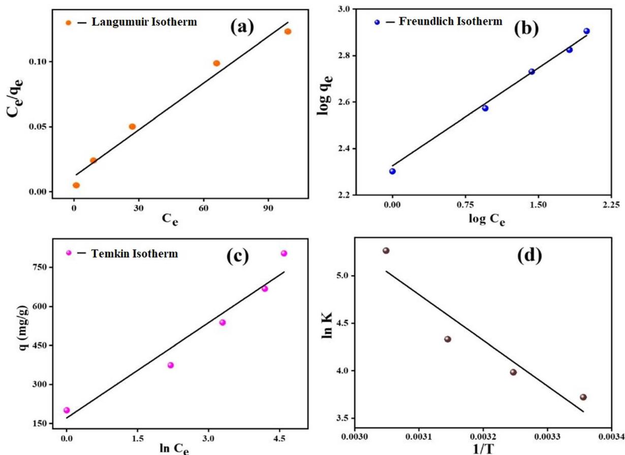
Fig. 5 Adsorption isotherms of the MgAl-LDH/LaFeO<sub>3</sub> composite: (a) Langmuir, (b) Freundlich, and (c) Temkin models. (d) Adsorption thermodynamics.
