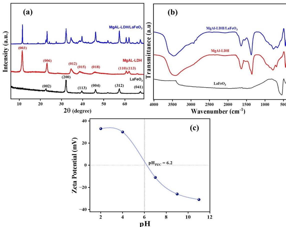
Fig. 1 XRD patterns (a) and FTIR spectra (b) for LaFeO<sub>3</sub>, MgAl-LDH and the MgAl-LDH/LaFeO<sub>3</sub> composite, and the zeta potential at different pH values (c) for the MgAl-LDH/LaFeO<sub>3</sub> composite.
