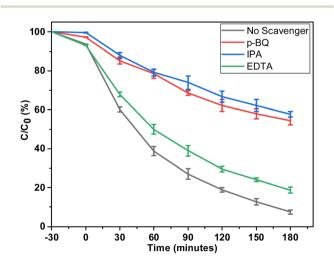
Fig. 3 Impact of different scavenging agents on the photocatalytic degradation of DCF on  $0.15 \text{CeO}_2/\text{g-C}_3 \text{N}_4$ .
