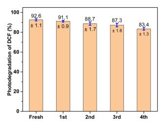
Fig. 6 Recyclability test of DCF photodegradation over  $0.15CeO_2/g-C_3N_4$  under visible light irradiation.
