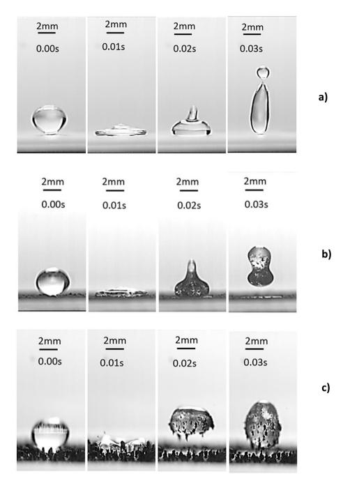
Fig. 4 High-speed camera images: (a) a droplet impacting on the hydrophobic surface, (b) a droplet impacting on the hydrophobic surface with loosely dispersed ferroparticles, and (c) a droplet impacting on the hydrophobic surface with loosely dispersed functionalized ferroparticles.
