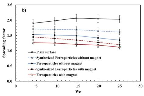
Fig. 5 (a) Contact time vs. Weber number for the different cases considered in the present study. (b) Spreading factor vs. Weber number for the different cases considered in the present study.
