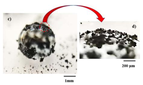
Fig. 2 (a) Functionalized ferroparticles floating on the water surface due to low surface free energy. (b) Immersion of as-received ferroparticles into water due to high surface free energy. (c) An optical image of functionalized ferroparticles attaching to the droplet surface. (d) An optical image showing a close-up view of functionalized ferroparticles attaching to the droplet surface.
