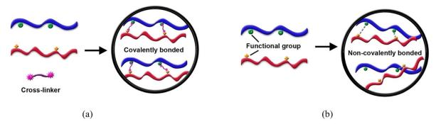
Fig. 7 Schematic illustration of polymer crosslinking mechanisms: (a) covalent bonding via cross-linkers and (b) non-covalent interactions via functional groups.<sup>135</sup> Ramachandran et al., Cross-linking dots on metal oxides, NPG Asia Mater., 2019, 11, 19, under the terms of the Creative Commons Attribution 4.0 International Licensee (https://creativecommons.org/licenses/by/4.0/).
