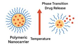
Fig. 16 Schematic illustration of thermo-responsive drug release: at temperatures below the LCST, the nanocarrier remains swollen and retains the drug; upon heating above the LCST, the polymer network collapses, triggering.
