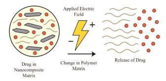
Fig. 18 Electro-responsive release mechanism.
