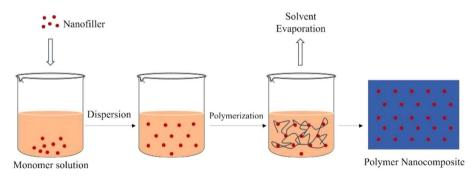
Fig. 9 Schematic representation of polymer nanocomposite fabrication *via in situ* polymerization.<sup>144</sup> Adopted from Basavegowda *et al.*, Advances in functional biopolymer-based nanocomposites for active food packaging applications, *Polymers*, 2021, **13**(23), 4198, under the terms of the Creative Commons Attribution 4.0 International License (https://creativecommons.org/licenses/by/4.0/).
