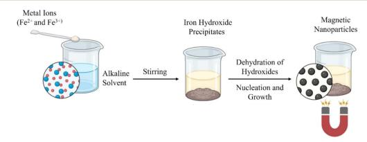
Fig. 14 Synthesis of magnetic nanoparticles. Synthesis of magnetic nanoparticles. Adopted from Stiufiuc *et al.*, Magnetic nanoparticles: synthesis, characterization, and their use in biomedical field, *Appl. Sci.*, 2024, 14(4), 1623, under the terms of the Creative Commons Attribution 4.0 International License (https://creativecommons.org/licenses/by/4.0/).
