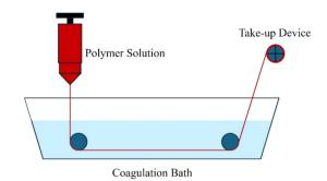
Fig. 12 Schematic representation of wet spinning procedure.
