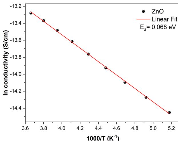
Fig. 9 Arrhenius plot of  $\ln \sigma_{AC}$  versus  $1000/T$  for ZnO NPs calcined at 500 °C, yielding an activation energy of 0.068 eV.
