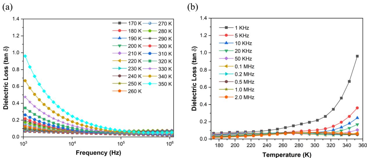
Fig. 6 (a) Dielectric loss ( $\tan \delta$ ) versus frequency for ZnO NPs calcined at 500 °C, recorded over the measurement temperature range of 170–350 K and (b) dielectric loss ( $\tan \delta$ ) versus temperature for ZnO NPs calcined at 500 °C, recorded over the measurement frequency range of  $10^3$  to  $10^6$  Hz.
