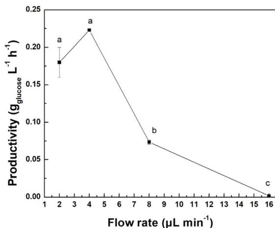
**Fig. 11** Effect of the flow rate on the productivity of cel@MbG microreactor. All analyses were conducted in triplicate, and the results are shown with the associated standard deviations (Table S11) (in some cases, the standard deviation was  $<0.001$ ; therefore, the error bars are not visible). Significant differences ( $p < 0.05$ ) among the different flow rates of the cel@MbG microreactor are represented by lowercase letters, using one-way ANOVA analysis.
