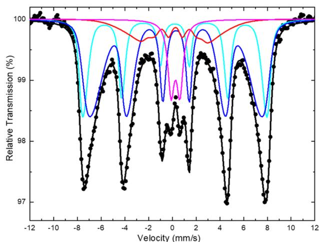
Fig. 5 <sup>57</sup>Fe Mössbauer spectrum of the MbG sample collected at room temperature. The points correspond to the experimental data, and the continuous lines to the components used to fit the spectrum.
