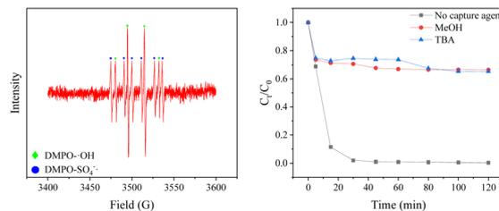
Fig. 7 EPR spectrum of DMPO capturing  $\cdot\text{OH}$  and  $\text{SO}_4^{\cdot-}$  at 15 minutes (a) and effects of different trapping agents on **SMX** degradation (b). (Conditions: initial concentration of **SMX** is 10  $\text{mg L}^{-1}$ , electrolyte  $\text{Na}_2\text{SO}_4$  concentration is 0.1  $\text{mol L}^{-1}$ , concentrations of MeOH and TBA are 0.1  $\text{mol L}^{-1}$ , current density is 0.08  $\text{mA cm}^{-2}$ ,  $\text{pH} = 7$ .)
