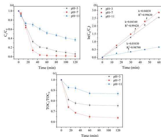
Fig. 3 Effect of pH on **SMX** degradation (a), quasi-first-order kinetic fitting (b), and TOC removal (c). (Conditions: initial concentration of **SMX** is  $10 \text{ mg L}^{-1}$ , electrolyte  $\text{Na}_2\text{SO}_4$  concentration is  $0.1 \text{ mol L}^{-1}$ , current density is  $0.08 \text{ mA cm}^{-2}$ )
