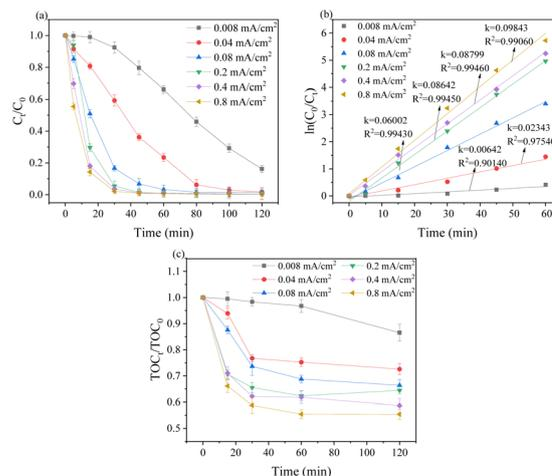
Fig. 2 Effect of current density on **SMX** degradation (a), quasi-first-order kinetic fitting (b), and TOC removal (c). (Conditions: initial concentration of **SMX** is  $10 \text{ mg L}^{-1}$ , electrolyte  $\text{Na}_2\text{SO}_4$  concentration is  $0.1 \text{ mol L}^{-1}$ , pH is not adjusted.)
