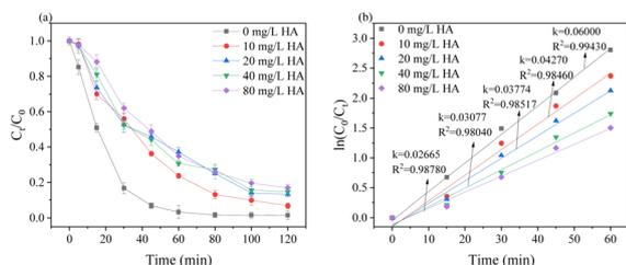
Fig. 6 Effect of HA on **SMX** degradation (a) and quasi-first-order kinetic fitting (b). (Conditions: initial concentration of **SMX** is 10  $\text{mg L}^{-1}$ , electrolyte  $\text{Na}_2\text{SO}_4$  concentration is 0.1  $\text{mol L}^{-1}$ , current density is 0.08  $\text{mA cm}^{-2}$ ,  $\text{pH} = 7$ .)
