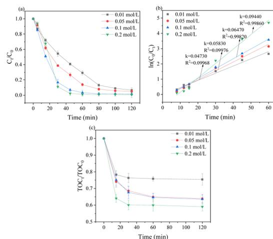
Fig. 4 Effect of electrolyte concentration on **SMX** degradation (a), quasi-first-order kinetic fitting (b) and TOC removal (c). (Conditions: initial concentration of **SMX** is  $10 \text{ mg L}^{-1}$ , current density is  $0.08 \text{ mA cm}^{-2}$ , pH = 7.)
