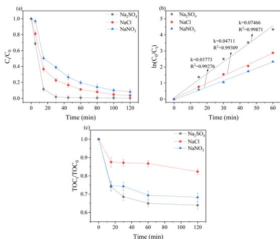
Fig. 5 Effect of electrolyte type on **SMX** degradation (a), quasi-first-order kinetic fitting (b), and TOC removal (c). (Conditions: initial concentration of **SMX** is  $10 \text{ mg L}^{-1}$ , current density is  $0.08 \text{ mA cm}^{-2}$ , pH = 7, electrolytes  $\text{Na}_2\text{SO}_4$ ,  $\text{NaCl}$  and  $\text{NaNO}_3$  are all  $0.1 \text{ mol L}^{-1}$ )
