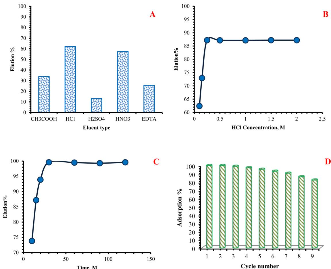
Fig. 12 (A) Effect of different eluting agents, (B) effect of HCl concentration, (C) effect of time on the desorption of cadmium from CDAM, and (D) recycling ability of CDAM for  $\text{Cd}^{2+}$  in consecutive nine cycles.
