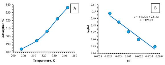
Fig. 11 (A) The effect of temperature on the sorption process of Cd<sup>+2</sup> ions upon CNT-AMP, (B) plot of log  $K_d$  vs. 1/T, of sorption of Cd<sup>+2</sup> ions upon CNT-AMP adsorbent. ([Cd<sup>+2</sup>] = 1700 ppm/20 mL, pH = 5.5, t = 45 minutes, 0.06 g dosage, T = 25 °C, agitation rate = 200 rpm]).
