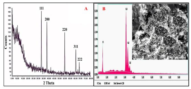
Fig. 14 (A) XRD, and (B) EDX, SEM, analysis of the produced CdO.
