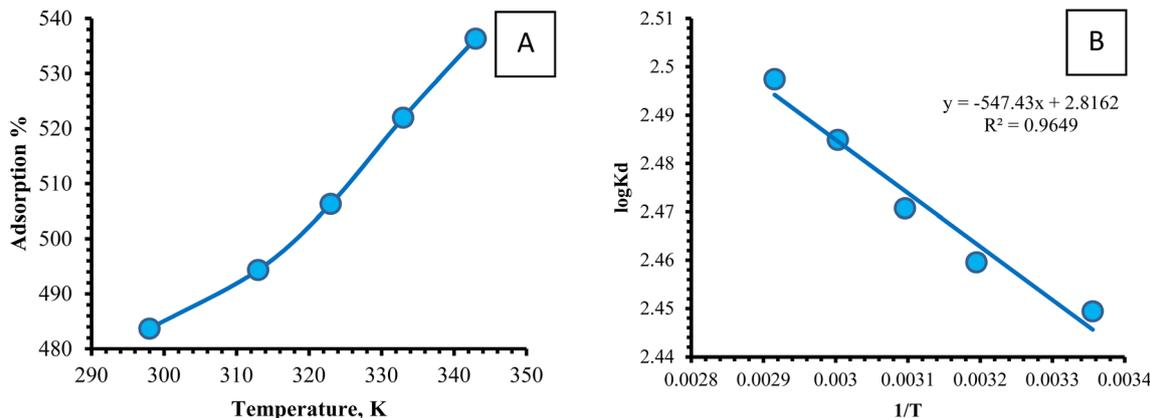
Fig. 11 (A) The effect of temperature on the sorption process of  $\text{Cd}^{2+}$  ions upon CNT-AMP, (B) plot of  $\log K_d$  vs.  $1/T$ , of sorption of  $\text{Cd}^{2+}$  ions upon CNT-AMP adsorbent. ( $[\text{Cd}^{2+}] = 1700 \text{ ppm}/20 \text{ mL}$ ,  $\text{pH} = 5.5$ ,  $t = 45 \text{ minutes}$ ,  $0.06 \text{ g}$  dosage,  $T = 25 \text{ }^\circ\text{C}$ , agitation rate =  $200 \text{ rpm}$ ).
