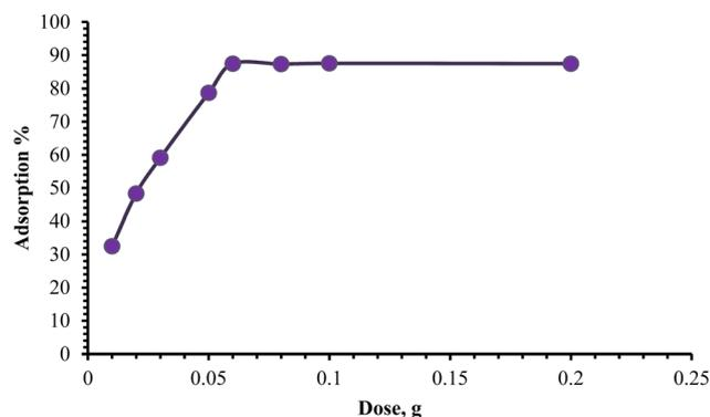
Fig. 8 The impact of adsorbent dose on the sorption process of  $\text{Cd}^{2+}$  by the CDAM.
