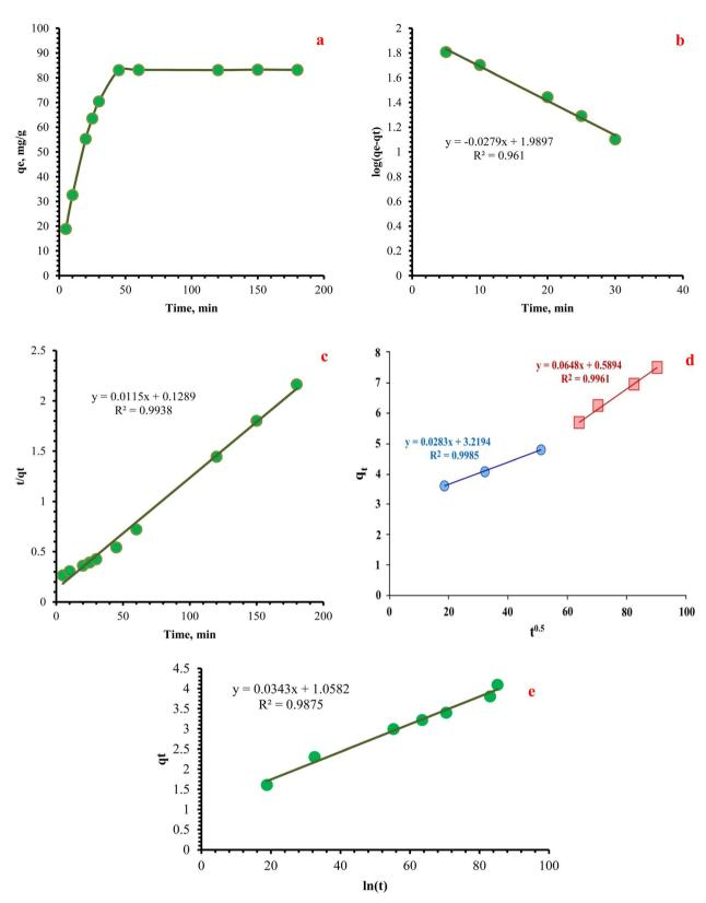
Fig. 9 (a) Time effect of the Cd<sup>+2</sup> adsorption, (b) pseudo 1st order, (c) pseudo 2nd order, (d) the IPD model, (e) Elovich model of Cd<sup>+2</sup> adsorption process using CDAM. ( $[Cd^{+2}] = 250 \text{ ppm/}20 \text{ mL}$ , pH = 5.5, t = 45 minutes, 0.06 g dosage,  $T = 25 \,^{\circ}\text{C}$ , agitation rate = 200 rpm]).
