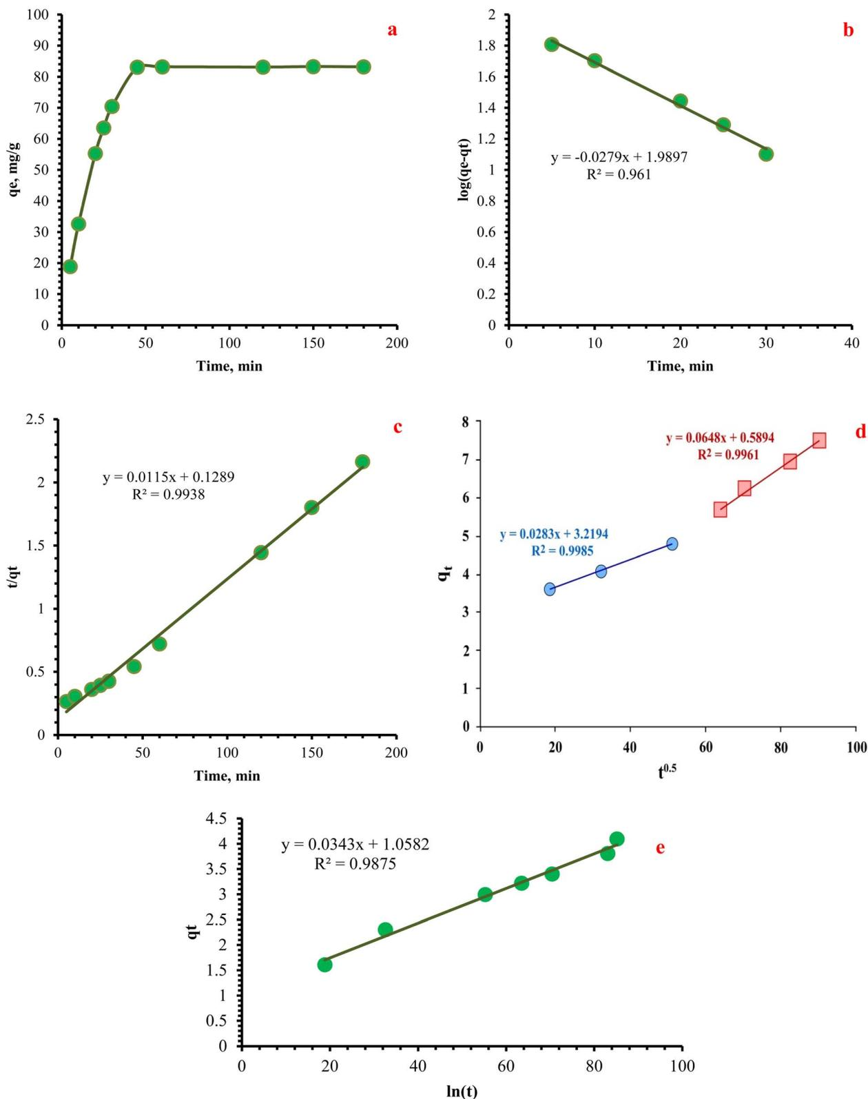
Fig. 9 (a) Time effect of the Cd<sup>2+</sup> adsorption, (b) pseudo 1st order, (c) pseudo 2nd order, (d) the IPD model, (e) Elovich model of Cd<sup>2+</sup> adsorption process using CDAM. ([Cd<sup>2+</sup>] = 250 ppm/20 mL, pH = 5.5, t = 45 minutes, 0.06 g dosage, T = 25 °C, agitation rate = 200 rpm).
