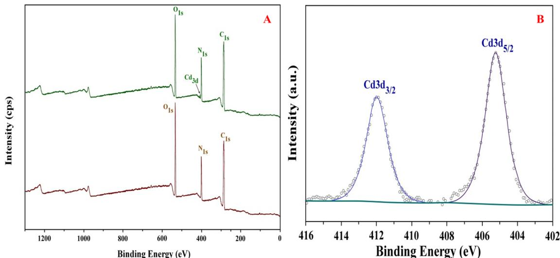
Fig. 3 XPS results of CDAM: (A) before and after sorption (full spectra) and (B) after the adsorption of Cd 3d.
