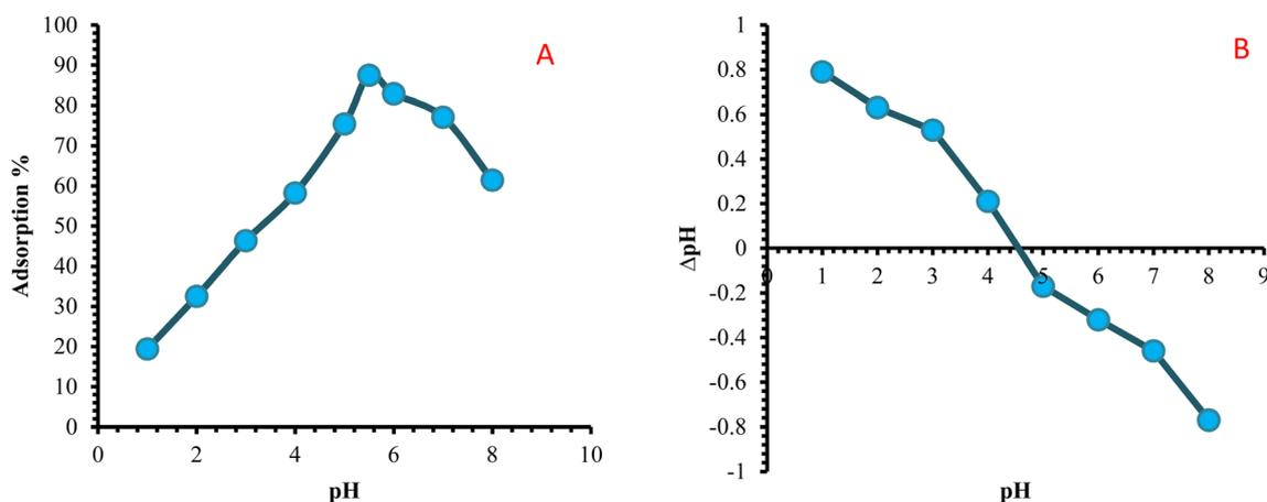
Fig. 7 (A) Impact of pH on the sorption of  $\text{Cd}^{+2}$  using CDAM, (B)  $\text{pH}_{\text{ZPC}}$  of the CDAM adsorbent.  $\text{Cd}^{+2}$  concentration, 250 mg L; CDAM dose 0.1 g; equilibration time, 20 min, and temperature, 30 °C.
