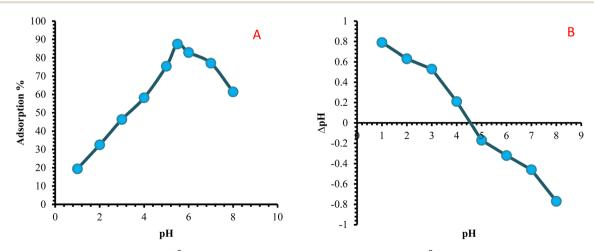
Fig. 7 (A) Impact of pH on the sorption of  $Cd^{+2}$  using CDAM, (B)  $pH_{ZPC}$  of the CDAM adsorbent.  $Cd^{+2}$  concentration, 250 mg L; CDAM dose 0.1 g; equilibration time, 20 min, and temperature, 30 °C.
