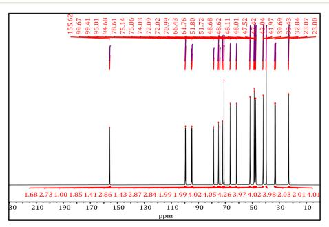
Fig. 5 13CNMR analysis of CDAM adsorbent
