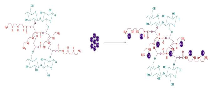
Scheme 2 Interaction mechanism between Cd<sup>2+</sup> ions and CDAM adsorbent.
