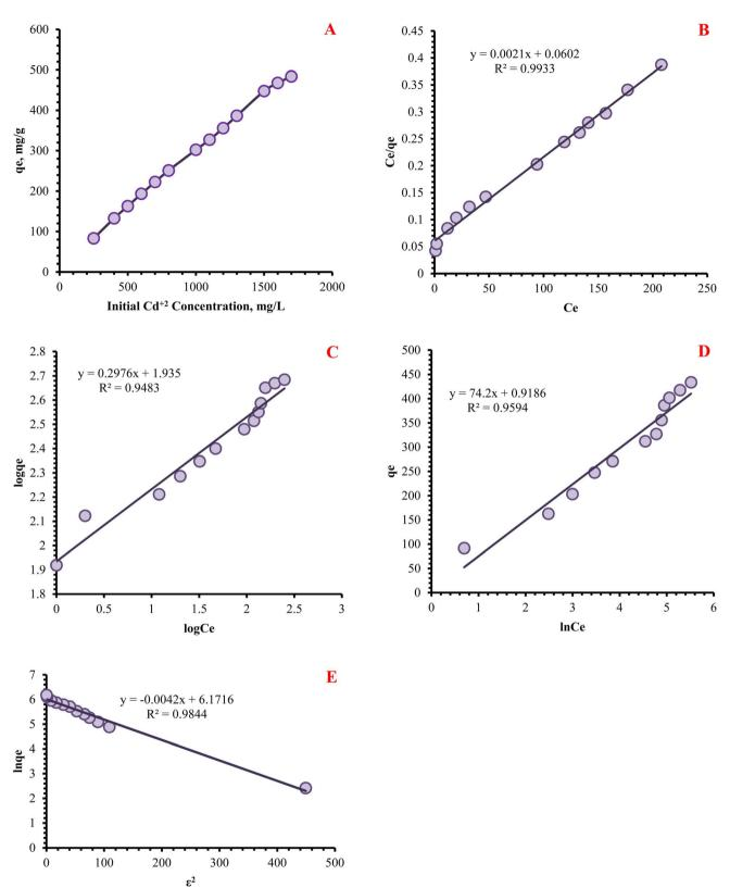
Fig. 10 (A) Initial cadmium concentration, (B) Langmuir, (C) Freundlich, (D) Tempkin, and (E) Dubinin-Radushkevich. Isotherm models of Cd<sup>+2</sup> ions adsorption using CDAM.
