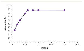
Fig. 8 The impact of adsorbent dose on the sorption process of  ${\rm Cd}^{+2}$  by the CDAM.
