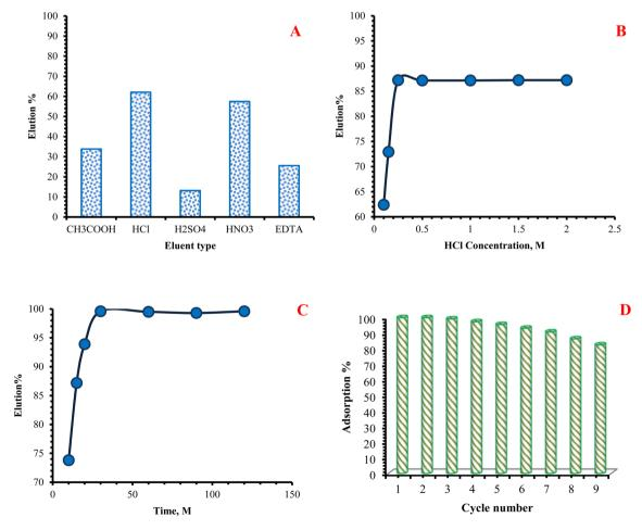
Fig. 12 (A) Effect of different eluting agents, (B) effect of HCl concentration, (C) effect of time on the desorption of cadmium from CDAM, and (D) recycling ability of CDAM for Cd<sup>2+</sup> in consecutive nine cycles.
