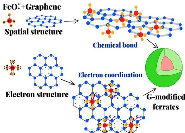
Fig. 1 Stability mechanism *via* electron balance and transfer in G-modified ferrates.
