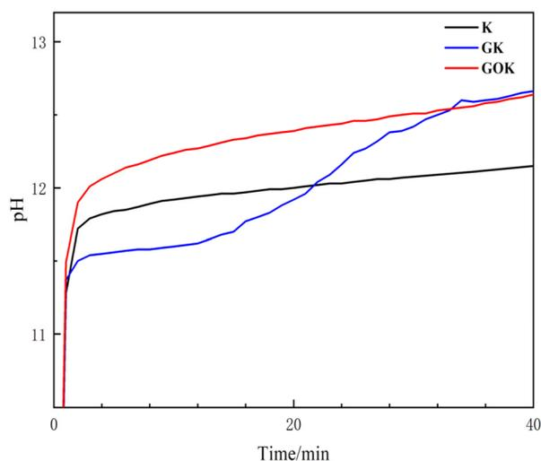
Fig. 3 pH changes during decomposition of unmodified and coated  $\text{K}_2\text{FeO}_4$  in water (K: unmodified  $\text{K}_2\text{FeO}_4$ ; GK: graphene-modified  $\text{K}_2\text{FeO}_4$ ; GO: GO-modified  $\text{K}_2\text{FeO}_4$ ).
