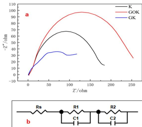
Fig. 6 (a) Electrochemical impedance spectroscopy (EIS) curves for unmodified (K), GO-modified ferrates (GOK), and graphene-modified ferrates (GK)  $K_2FeO_4$ ; (b) simulated equivalent circuit diagram.
