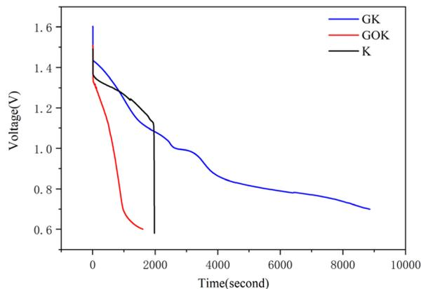
Fig. 5 Constant resistance discharge curves (200  $\Omega$  load) for coin cells with cathodes of: graphene-modified  $K_2FeO_4$  (GK), GO-modified  $K_2FeO_4$  (GOK), and unmodified  $K_2FeO_4$  (K).
