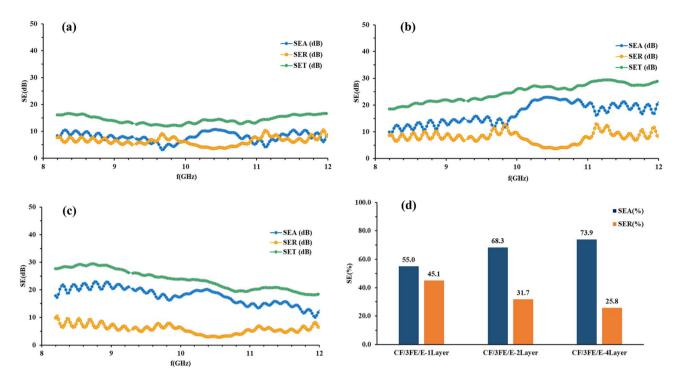
Fig. 12  $SE_{A}$ ,  $SE_{R}$ , and  $SE_{T}$  of (a) CF/3FE/E single-layer, (b) CF/3FE/E double-layer, (c) CF/3FE/E four-layer composites, and (d) the corresponding  $SE_{A}$  and  $SE_{R}$  percentage contributions for all CF/3FE/E samples.
