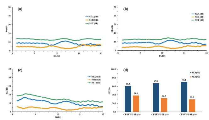
Fig. 10 SE<sub>A</sub>, SE<sub>B</sub>, and SE<sub>T</sub> of (a) CF/1FE/E single-layer, (b) CF/1FE/E double-layer, (c) CF/1FE/E four-layer composites, and (d) the corresponding SE<sub>A</sub> and SE<sub>B</sub> percentage contributions for all CF/1FE/E samples.
