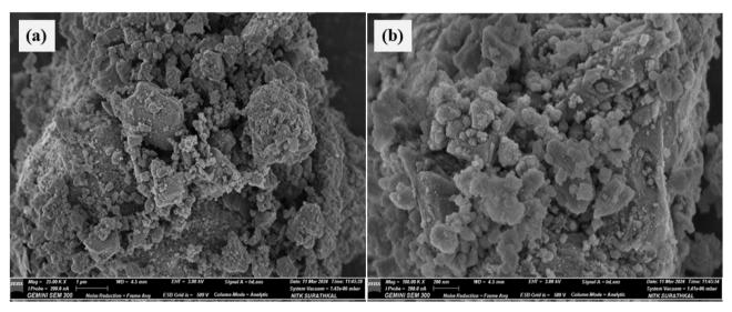
Fig. 4 FESEM images of Fe<sub>2</sub>O<sub>3</sub> nano filler at (a)  $25\,000\times$  and (b)  $100\,000\times$  magnification.
