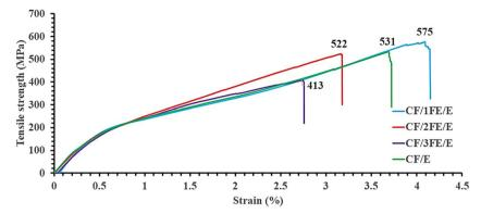
Fig. 7 Tensile behaviour of carbon fabric and Fe<sub>2</sub>O<sub>3</sub> reinforced epoxy (CF/FE/E) composites
