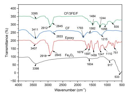
Fig. 6 FTIR spectra of Fe<sub>2</sub>O<sub>3</sub> nanoparticles, epoxy, carbon fabric and carbon fabric/Fe<sub>2</sub>O<sub>3</sub>/epoxy (CF/3FE/F) composite.
