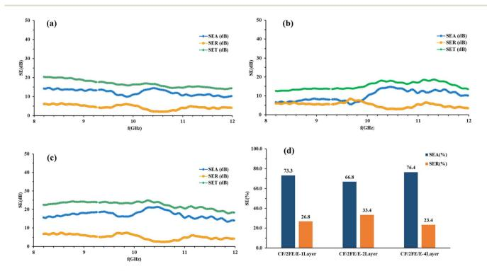
Fig. 11 SE<sub>A</sub>, SE<sub>R</sub>, and SE<sub>T</sub> of (a) CF/2FE/E single-layer, (b) CF/2FE/E double-layer, (c) CF/2FE/E four-layer composites, and (d) the corresponding  ${\sf SE}_{\sf A}$  and  ${\sf SE}_{\sf R}$  percentage contributions for all CF/2FE/E samples.
