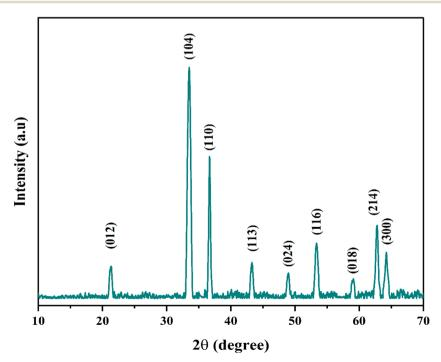
Fig. 5 X-RD spectra of Fe<sub>2</sub>O<sub>3</sub> nanoparticles.
