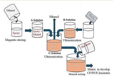
Fig. 2 Fe<sub>2</sub>O<sub>3</sub>-filled epoxy matrix preparation.
