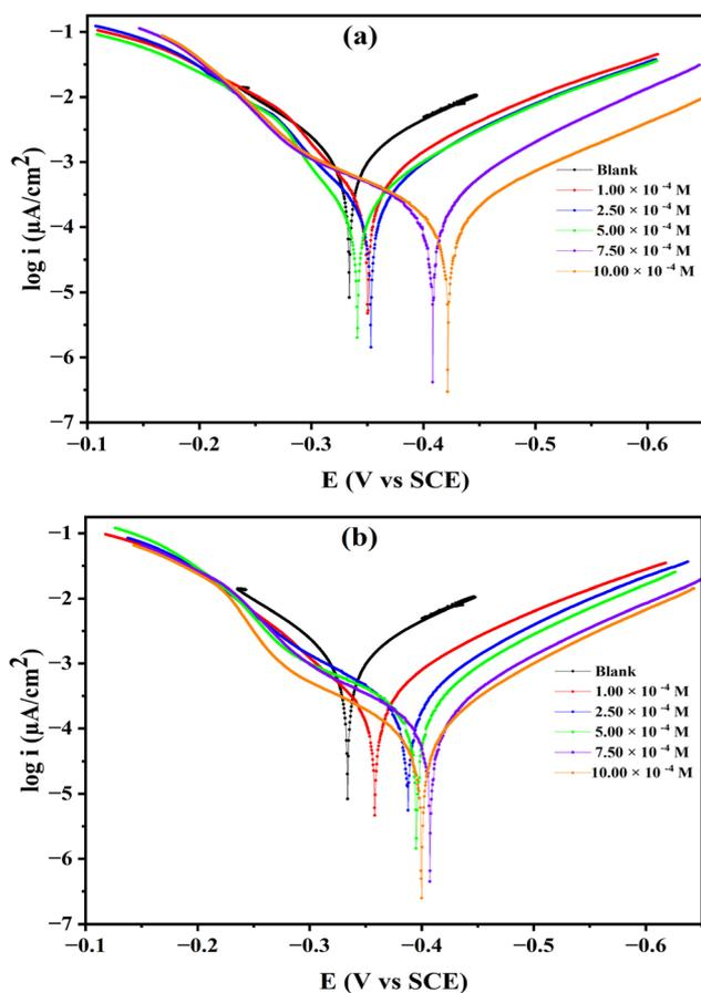
Fig. 1 Potentiodynamic polarization curves for the corrosion of carbon steel in 1.0 M HCl in absence and presence of different concentrations of Rhamnose (a) and Salicin (b) compounds at  $30^\circ\text{C}$ .
