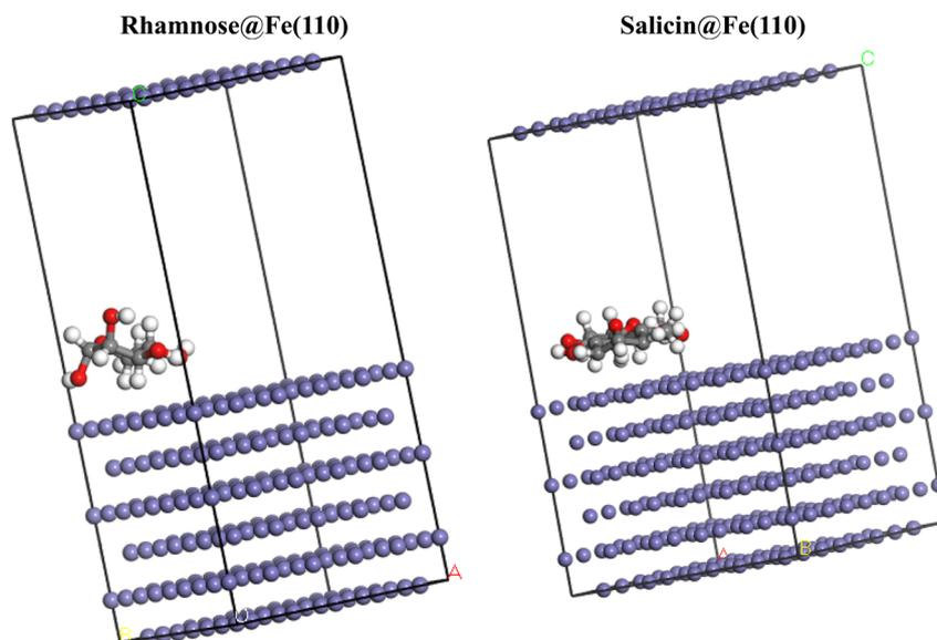
Fig. 6 Favorable configurations of Rhamnose@Fe(110) and Salicin@Fe(110) complexes.
