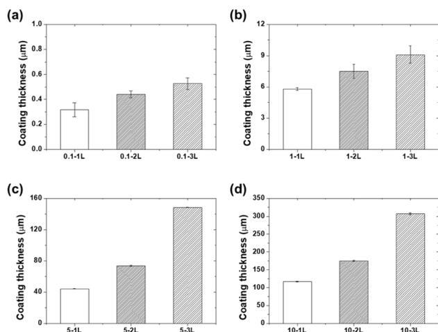
Fig. 4 Coating thickness as a function of the mold fill level for (a) 0.1 wt%, (b) 1 wt%, (c) 5 wt%, and (d) 10 wt% PVA concentrations.
