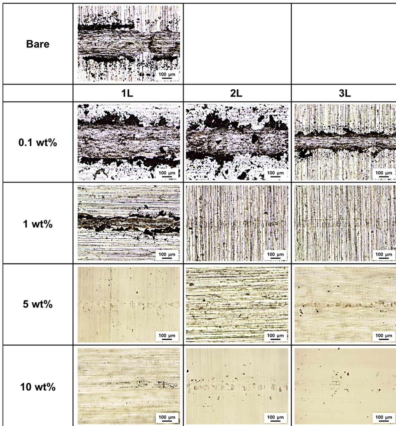
Fig. 8 Optical microscopy images of wear tracks after 5000 cycles at a 50 mN load.
