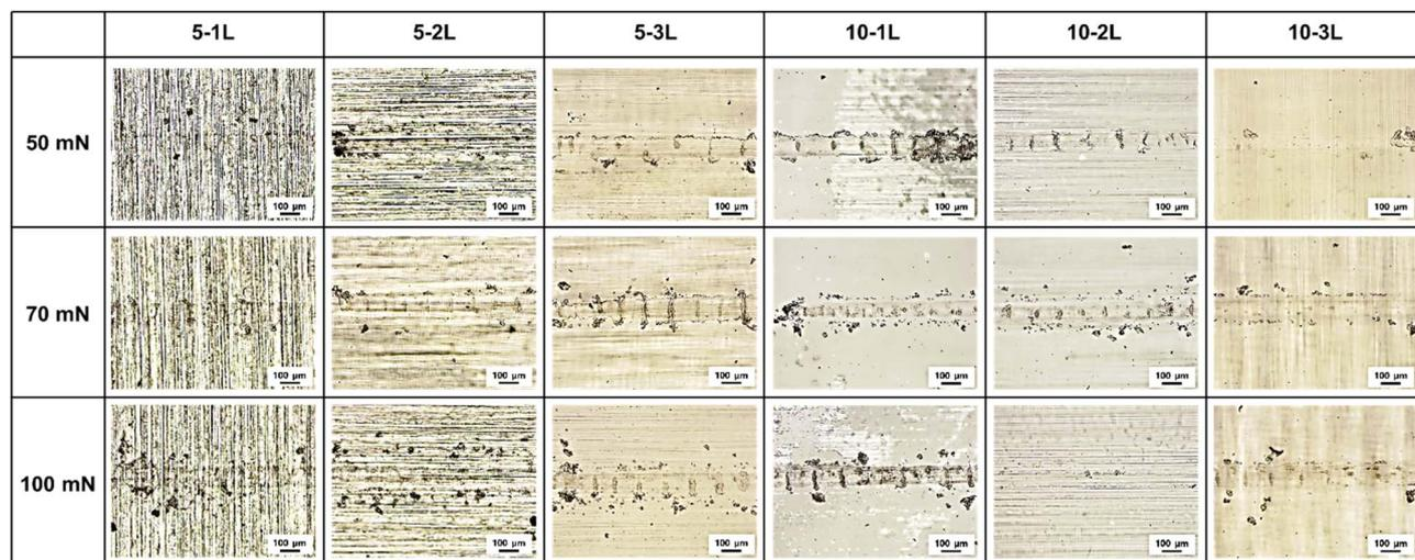
Fig. 10 Optical microscopy images of wear tracks for selected coatings under different loads after 10 000 cycles.
