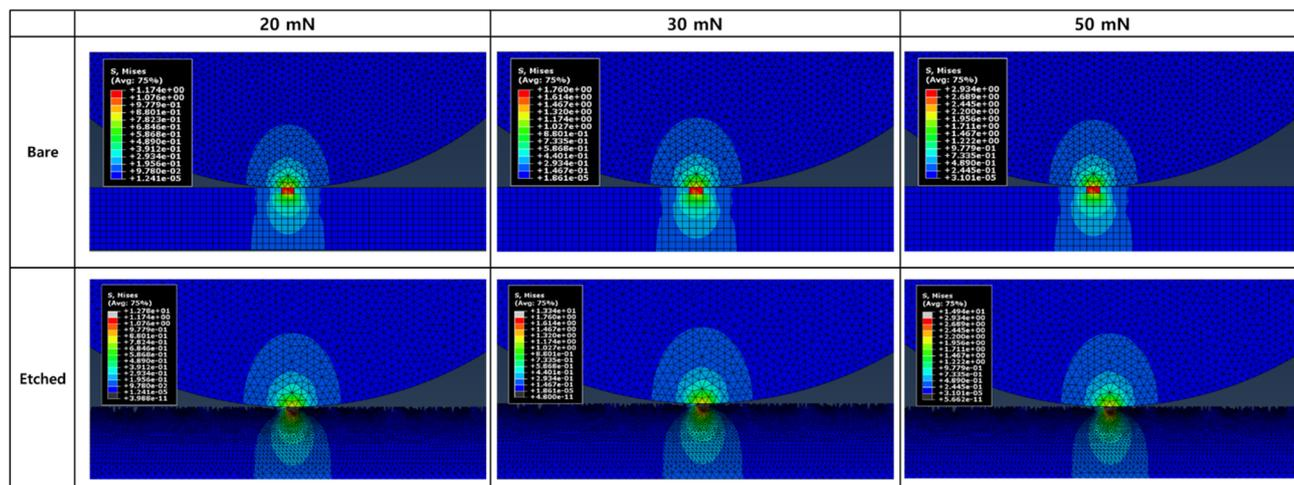
Fig. 11 Finite element analysis (FEA) simulation results of stress distribution in bare glass and etched glass during indentation under different normal loads.
