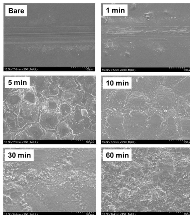
Fig. 8 Scanning electron microscopy images of wear tracks formed on glass samples after sliding tests.
