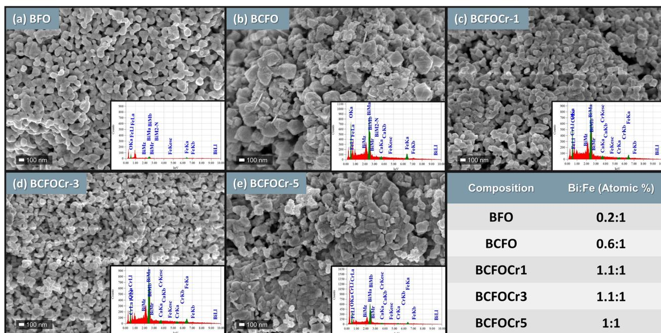
Fig. 3 SEM image of (a) BFO, (b) BCFO, (c) BCFOCr1, (d) BCFOCr3, and (e) BCFOCr5 with their insets showing representative EDS spectra from a single characteristic point.
