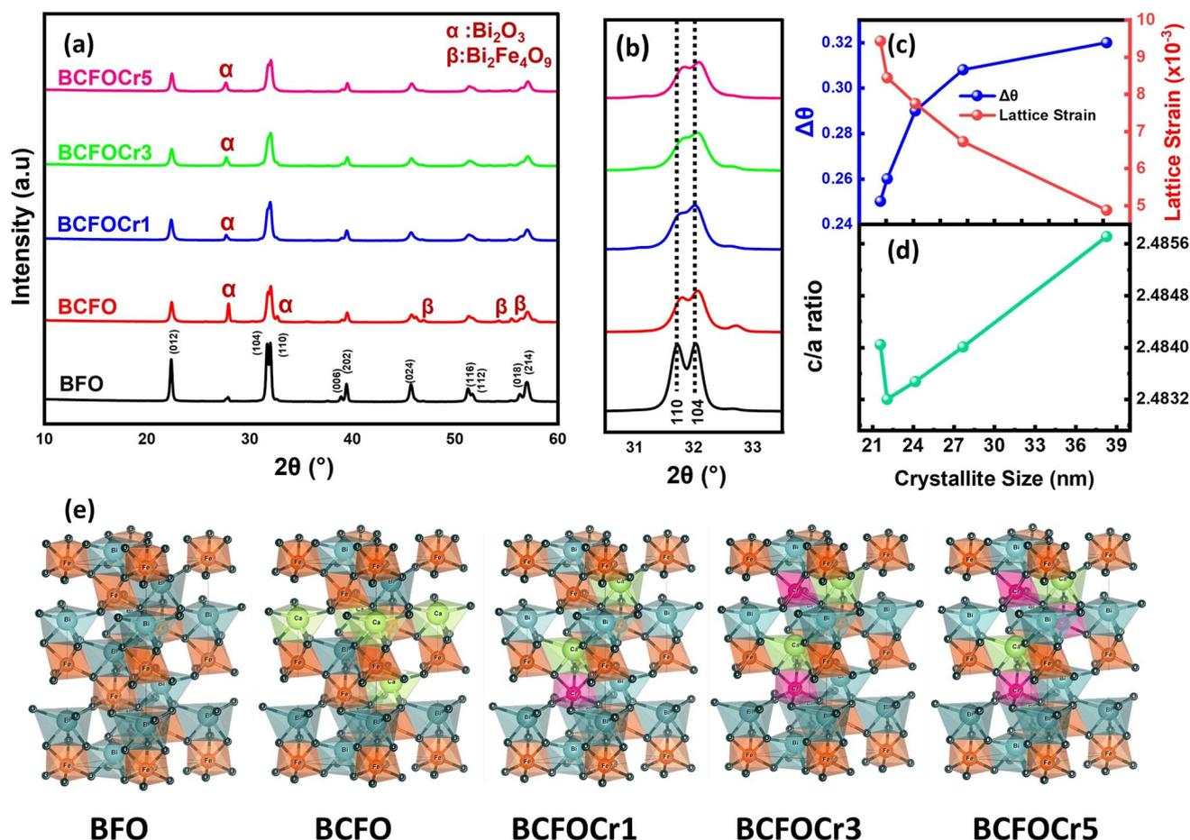
Fig. 2 (a) XRD analysis of all compositions showcasing the major peaks (b) narrow  $2\theta$  region of the major diffraction peak showing broadening upon dopant incorporation (c)  $\Delta\theta$  and lattice strain vs. crystallite size (d)  $c/a$  ratio vs. crystallite size (e) crystal structures of all synthesized compositions.
