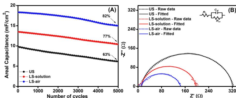
Fig. 7 (A) Capacitance retention at different numbers of cycles and (B) Nyquist plot of the US, LS-solution and LS-air samples recorded in 1 M KOH; (inset) corresponding circuit used to fit EIS data.
