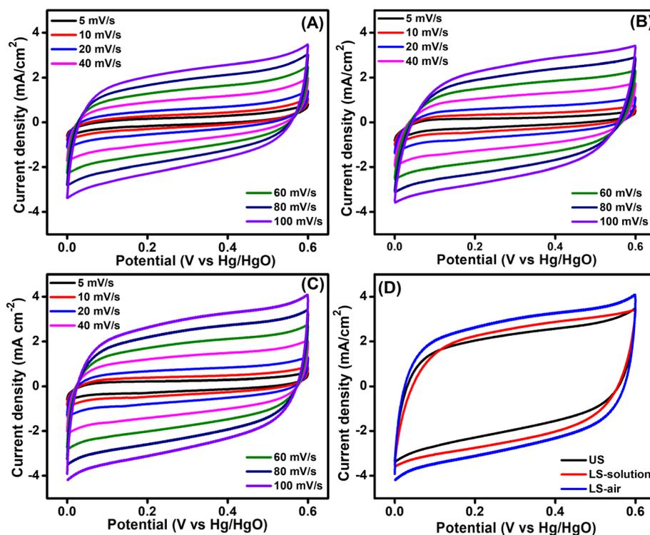
Fig. 5 CV curves of (A) US, (B) LS-solution, (C) LS-air current collectors at different scan rates from 5 to 100 mV s<sup>-1</sup> and (D) comparative CV curves at 100 mV s<sup>-1</sup> scan rate for all the samples in 1 M KOH.
