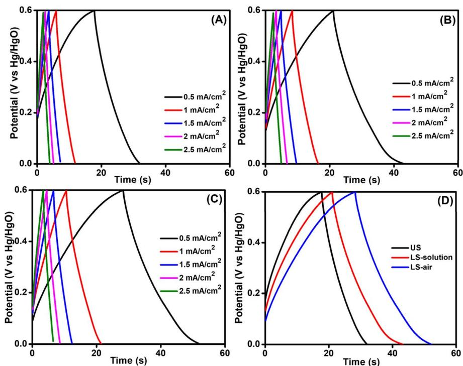
Fig. 6 GCD curves of (A) US, (B) LS-solution, (C) LS-air current collectors at different current densities from 0.5 to 2.5 mA cm<sup>-2</sup> and (D) comparative GCD curves at 0.5 mA cm<sup>-2</sup> current density for all the samples in 1 M KOH.
