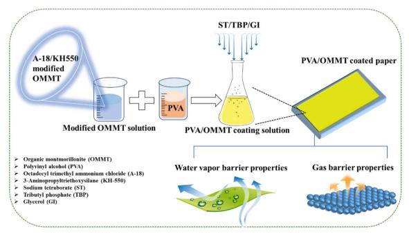
Fig. 1 A schematic diagram of the PVA/OMMT composite coating and coated paper preparation process.
