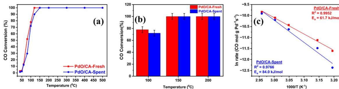
Fig. 5 (a) Light-off temperature, (b) comparative activities at three temperatures, and (c) activation energy of PdO/CA-fresh and PdO/CA-spent catalysts for CO oxidation. Conditions: GHSV 90 000 ( $\text{cc g}_{\text{cat}}^{-1} \text{h}^{-1}$ ); 1 h reaction time at each temperature to reach a steady state.
