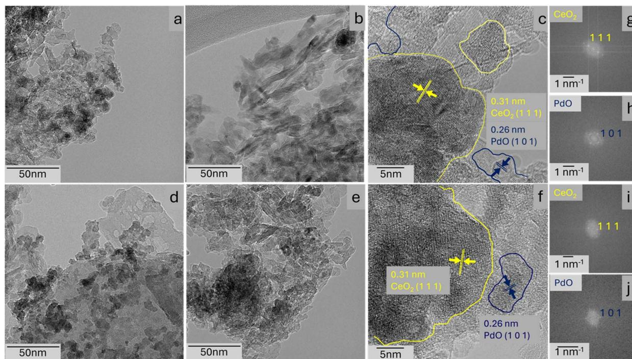
Fig. 3 HRTEM Ceta images of PdO/CA-fresh (a–c) and PdO/CA-spent (d–f) catalysts, displaying their morphologies: (c and f) lattice fringes and crystal planes in the crystallites of PdO and CeO<sub>2</sub> in 5 nm Ceta HRTEM images; (g–j) FFT patterns of (c and f).
