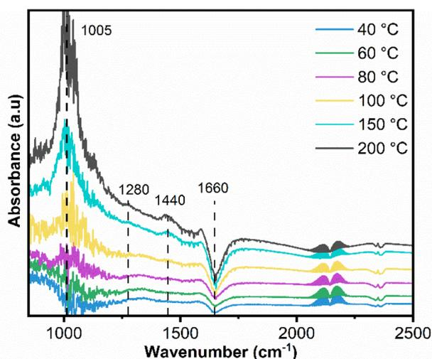
Fig. 8 *In situ* DRIFTS spectra of the dual support (CeO<sub>x</sub>/Al<sub>2</sub>O<sub>3</sub>). The *in situ* DRIFTS experiment was conducted in the gas cell by degassing in argon at 150 °C and cooling to 40 °C; 25 SCCM of 1% CO/4% O<sub>2</sub>/N<sub>2</sub> was introduced into the cell for 15 min to equilibrate, and then, a spectrum was recorded. The procedure was repeated at 40–200 °C.
