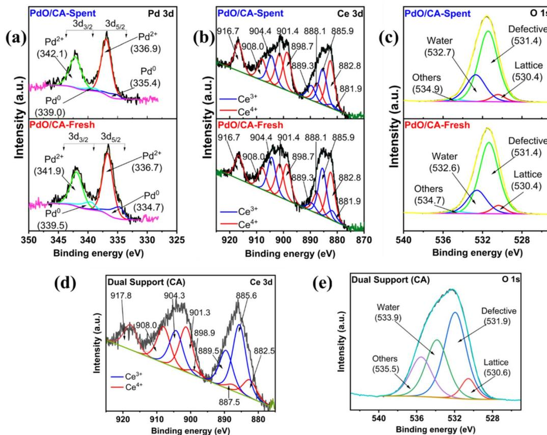
Fig. 4 Curve fitted (a) Pd 3d, (b) Ce 3d, and (c) O 1s X-ray core level spectra for the catalyst samples and (d) Ce 3d and (e) O 1s for the support.
