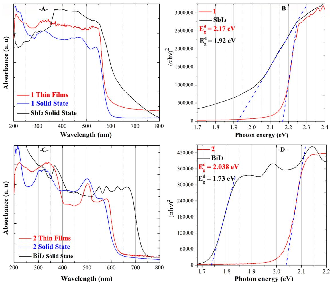
Fig. 10 (A and C) UV-vis absorption spectra of **1**, **2**,  $\text{SbI}_3$  and  $\text{BiI}_3$  as thin films and powder samples. (B and D) Tauc plot for direct band gap spectra of crystallized films for **1**, **2**,  $\text{SbI}_3$  and  $\text{BiI}_3$  taken at room temperature;  $\alpha$  is the absorption coefficient.
