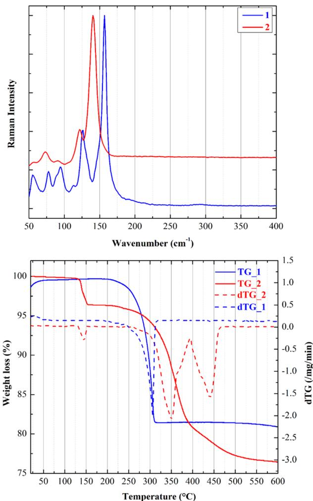
Fig. 8 (Top) Raman spectra of **1** and **2** recorded in the low-frequency range. (Bottom) The TG/DTG spectra of **1** and **2**.
