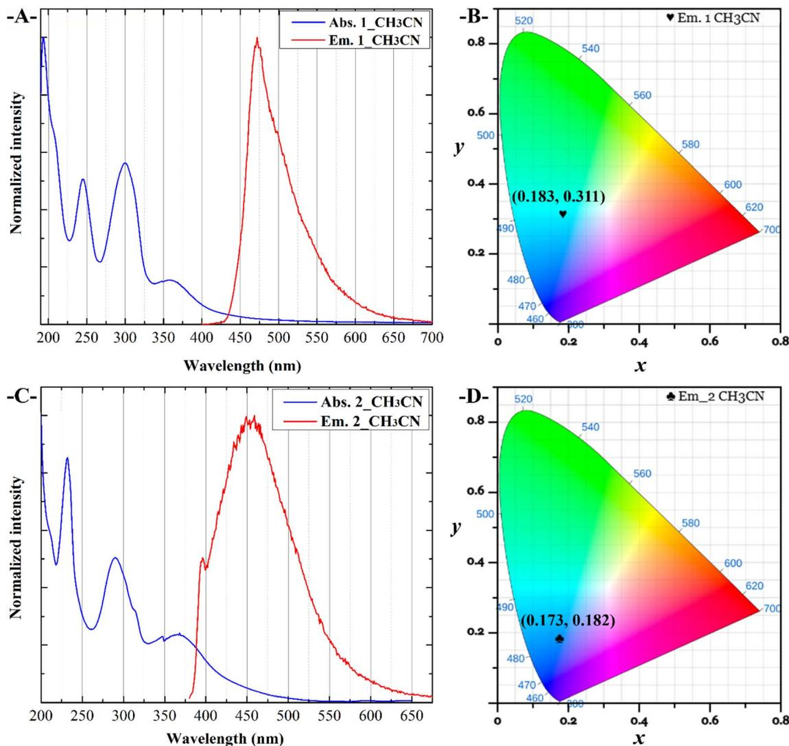
Fig. 9 Normalized absorption and emission spectra of compounds 1 (A) and 2 (C) recorded in CH<sub>3</sub>CN at 298 K. Commission Internationale de l'Eclairage (CIE) chromaticity coordinates of 1 (B) and 2 (D) at 298 K.
