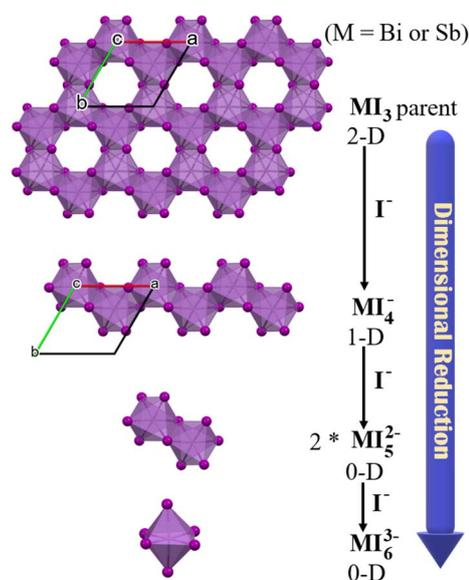
Fig. 2 Anionic networks, [MI<sub>4</sub>]<sup>-</sup>, [M<sub>2</sub>I<sub>10</sub>]<sup>4-</sup> and [MI<sub>6</sub>]<sup>3-</sup>, derived from the parent BiI<sub>3</sub>/SbI<sub>3</sub> (2-D) compounds, illustrating the concept of dimensional reduction.
