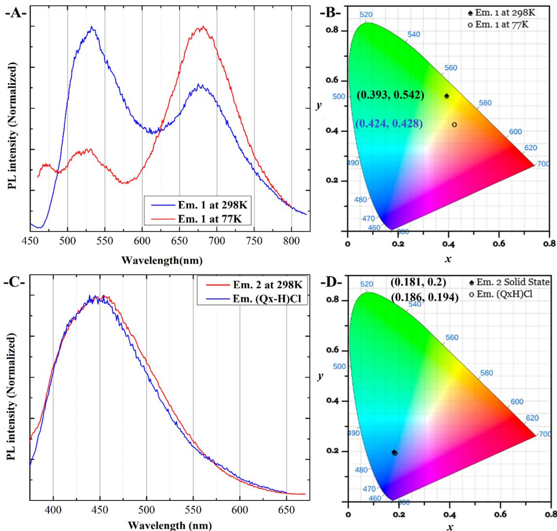
Fig. 11 (A) Normalized solid-state emission spectra **1** recorded at 298 K (blue) and 77 K (red). (B) Commission Internationale de l'Eclairage (CIE) chromaticity coordinates of **1** at 298 K and 77 K. (C) Normalized emission spectra of **2** (red) and (Qx-H)Cl (blue) recorded in solid-state at 298 K. (D) CIE chromaticity coordinates of **2** and (Qx-H)Cl at 298 K.
