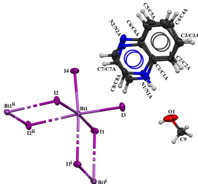
Fig. 5 The asymmetric part of the unit cell of crystals **2**, showing the atom-numbering scheme. Dashed lines represent bonds to adjacent symmetry-generated atoms (symmetry codes: (i)  $-x + 1, -y + 2, -z + 1$ ; (ii)  $-x, -y + 2, -z + 1$ ). Displacement ellipsoids are drawn at the 50% probability level and H atoms as small spheres of arbitrary radii.
