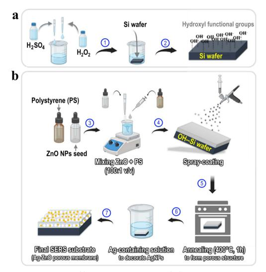
Fig. 1 (a) Piranha treatment silicone substrates. (b) Illustrating synthesis process of Ag/ZnO porous membrane on silicon wafer.
