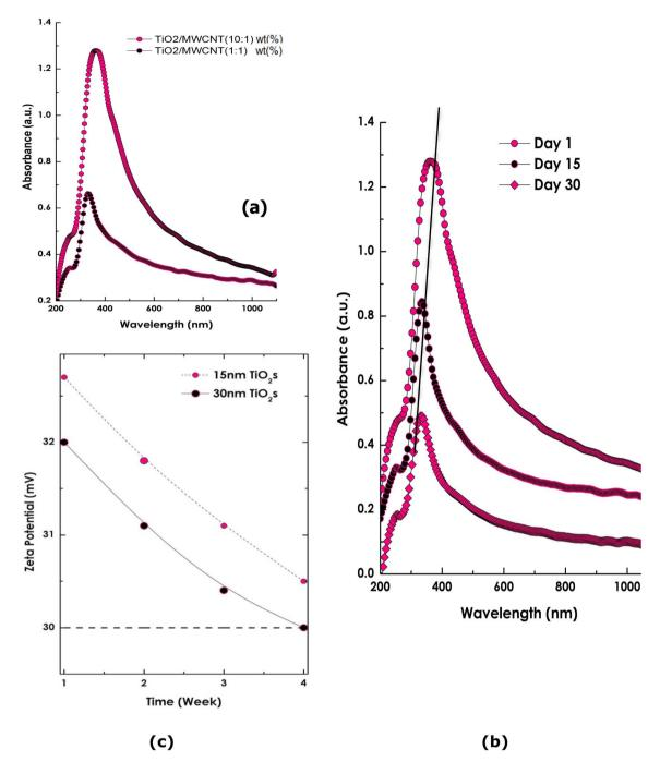
Fig. 6 (a) Optical absorbance spectra of  $TiO_2/MWCNT$ -EG nanofluids at different  $TiO_2$  loadings (MWCNT:  $TiO_2 = 10:1$  and 1:1 wt%) using 15 nm  $TiO_2$ . (b) Time-evolution of the optical spectra for  $TiO_2$  (15 nm)/MWCNT-EG (1:1 wt%) measured on days 1, 15, and 30. (c) Variation of zeta potential over time for 15 nm and 30 nm  $TiO_2/MWCNT$ -EG hybrid nanofluids.
