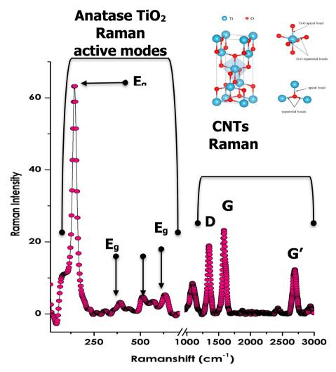
Fig. 5 Raman spectrum of TiO<sub>2</sub>/MWCNT (15 nm) nanocomposite at room temperature
