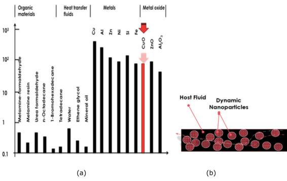
Fig. 1 (a) Comparative scale of thermal conductivities of organic materials, standard heat-transfer fluids, and metallic/oxide solids. (b) Schematic representation of a nanofluid comprising suspended nanoparticles in a host fluid.
