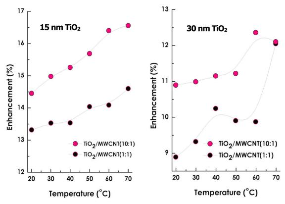
Fig. 8 Thermal conductivity enhancement of the optimized TiO<sub>2</sub> (15 nm, 30 nm/0.01 & 0.001 wt%)/MWCNTs (0.001wt%) nano fluids.
