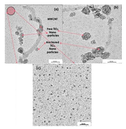
Fig. 4 Transmission electron microscopy (TEM) images of  $TiO_2$ -decorated MWCNT/EG hybrid nanofluids: (a) 15 nm  $TiO_2$ , (b) 30 nm  $TiO_2$ , and (c) magnified region of 15 nm  $TiO_2$ .
