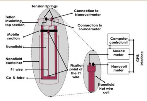
Fig. 3 Schematic representation of the transient hot-wire setup used for thermal conductivity measurements.
