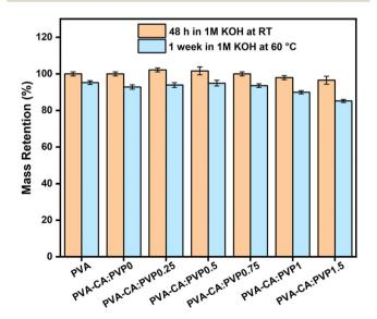
Fig. 7 Mass retention of the produced ISMs after 48 hours in  $1\,\mathrm{M}$  KOH at room temperature and after  $1\,\mathrm{week}$  in  $1\,\mathrm{M}$  KOH at  $60\,\mathrm{^{\circ}C}$ .
