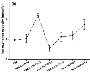
Fig. 11 (a)  ${\sf OH}^-$  ionic conductivity and (b) ion exchange capacity of the prepared membranes.
