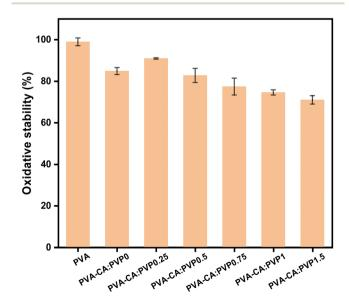
Fig. 10 Oxidative Stability of the ion-solvating membranes.
