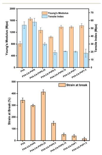
Fig. 13 Mechanical properties of the prepared ion-solvating membranes.
