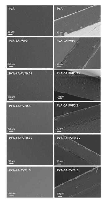
Fig. 5 Top and cross-sectional views of the prepared ion-solvating membranes
