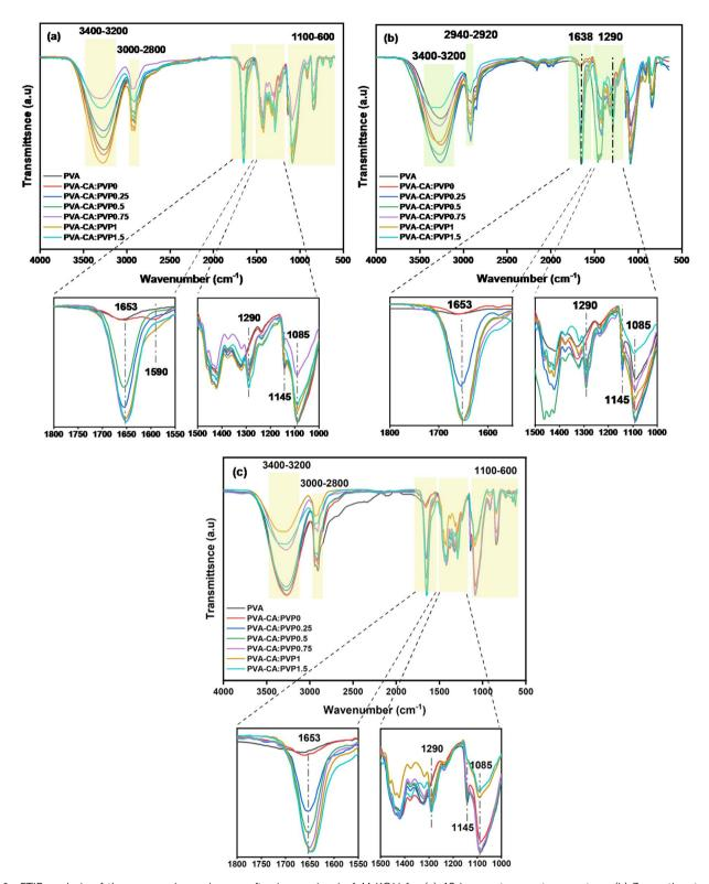
Fig. 9 FTIR analysis of the prepared membranes after immersion in 1 M KOH for (a) 48 hours at room temperature, (b) 3 months at room temperature and (c) 1 week at 60  $^{\circ}$ C.
