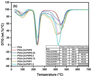
Fig. 12 Thermal stability of the produced ion-solvating membranes. (a) ATG curve, (b) DTG curve.
