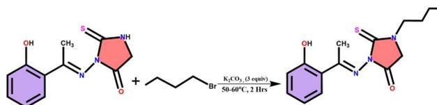
Scheme 7 Synthesis of (*E*)-1-butyl-3-((1-(2-hydroxyphenyl)ethylidene)amino)-2-thioxoimidazolidin-4-one.
