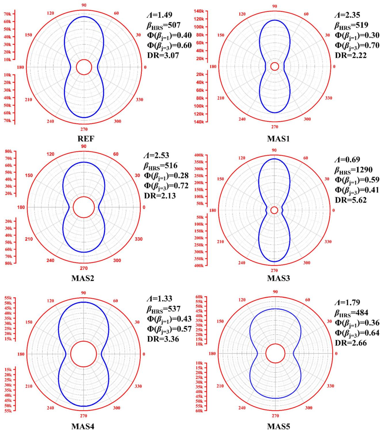
Fig. 11 The polar representation of harmonic light intensities versus polarization angle  $\omega$  at  $\lambda =$  infinite wavelength.
